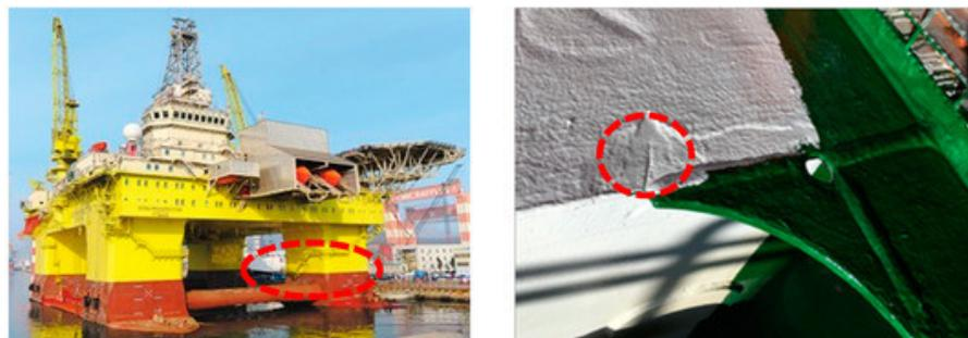
Figure 4. Crack at weld seam of offshore platform [9].
