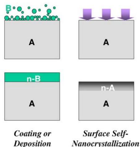
**Figure 2.** Schematic illustrations of (A) surface coating and (B) surface nano-crystallization reprinted with permission from Ref. [13]. Copyright 2022, ELSEVIER.
