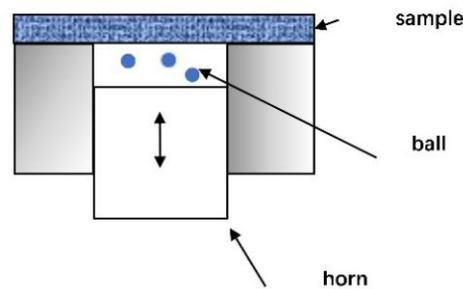
**Figure 4.** Schematic illustrations of the USSP process.
