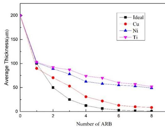
**Figure 15.** Variations of layer thickness versus the number of ARB passes reprinted with permission from Ref. [50]. Copyright 2022, ELSEVIER.
