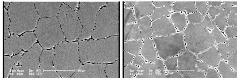
**Figure 13.** Microstructures of the conventional (left) and ultrasonic (right) ECAP-processed pure Al reprinted with permission from Ref. [47]. Copyright 2022, ELSEVIER.
