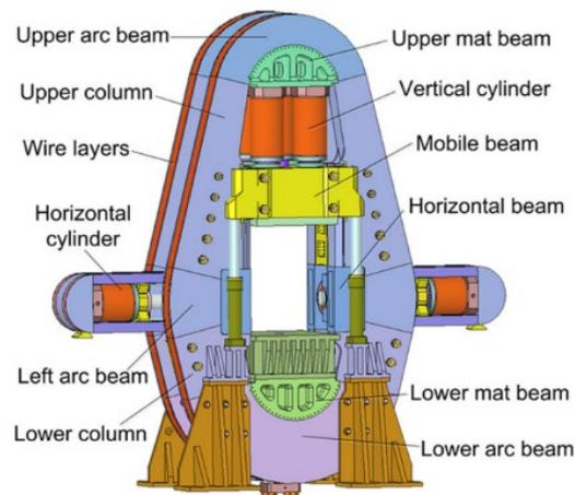
**Figure 17.** The main structure of MDF reprinted with permission from Ref. [58]. Copyright 2022, ELSEVIER.
