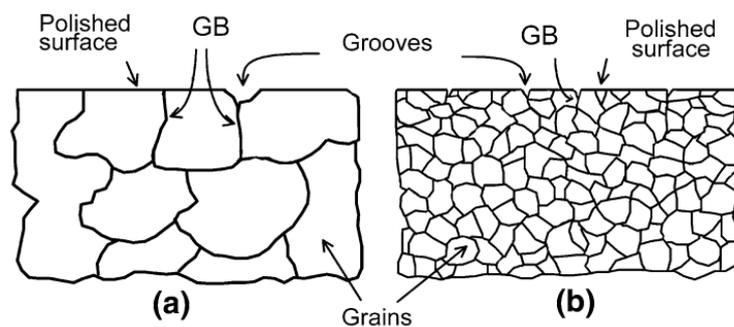
**Figure 19.** Schematic illustration of the presence of grooves on polished (a) coarse-grained and (b) nano-grained surfaces reprinted with permission from Ref. [79]. Copyright 2022, Springer.
