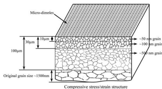
**Figure 8.** Schematic illustration of structure characteristics and distributions in a surface layer subjected to the UNSM reprinted with permission from Ref. [31]. Copyright 2022, ELSEVIER.
