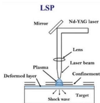
**Figure 5.** Schematic illustration of the LSP process reprinted with permission from Ref. [23]. Copyright 2022, Marketplace.
