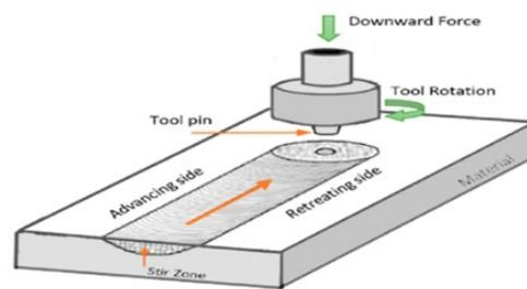
**Figure 6.** Schematic illustrations of the friction stir process reprinted from [26].
