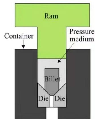
**Figure 16.** Schematic diagrams of hydrostatic extrusion reprinted with permission from Ref. [54]. Copyright 2022, ELSEVIER.
