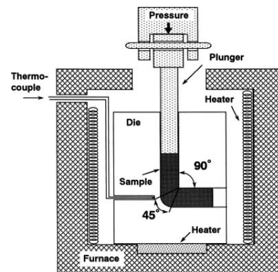
**Figure 10.** Schematic illustration of the ECAP reprinted with permission from Ref. [34]. Copyright 2022, ELSEVIER.
