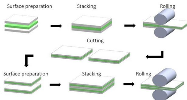
**Figure 14.** Diagrammatic representation of the accumulative roll-bonding (ARB) process reprinted with permission from Ref. [49]. Copyright 2022, ELSEVIER.
