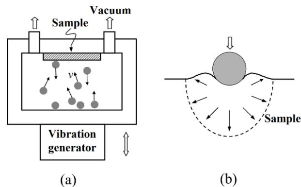
**Figure 3.** Schematic illustrations of the (a) SMAT setup and (b) localized plastic deformation in the surface layer of the treated sample, caused by the impact of balls reprinted with permission from Ref. [19]. Copyright 2022, ELSEVIER.
