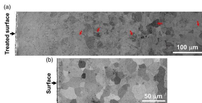
**Figure 20.** Cross-sectional scanning electron microscope (SEM) images of (a) gradient nanostructured surface (GNS) Ti samples and (b) coarse-grained (CG) Ti samples reprinted with permission from Ref. [17]. Copyright 2022, WILEY.
