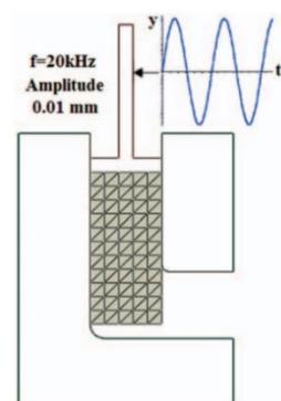
**Figure 12.** Applying ultrasonic vibration onto the plunger during the ECAP process reprinted with permission from Ref. [46]. Copyright 2022, ELSEVIER.
