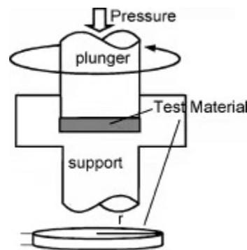
**Figure 9.** Schematic illustrations of the high-pressure torsion process reprinted with permission from Ref. [34]. Copyright 2022, ELSEVIER.
