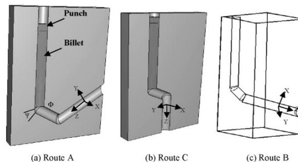
**Figure 11.** FEM (finite element method) models of ECAP reprinted with permission from Ref. [41]. Copyright 2022, ELSEVIER.
