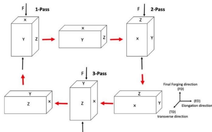
**Figure 18.** Process of MDF reprinted with permission from Ref. [59]. Copyright 2022, ELSEVIER.
