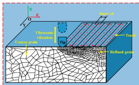
**Figure 7.** Schematic illustration of the UNSM process reprinted with permission from Ref. [29]. Copyright 2022, ELSEVIER.
