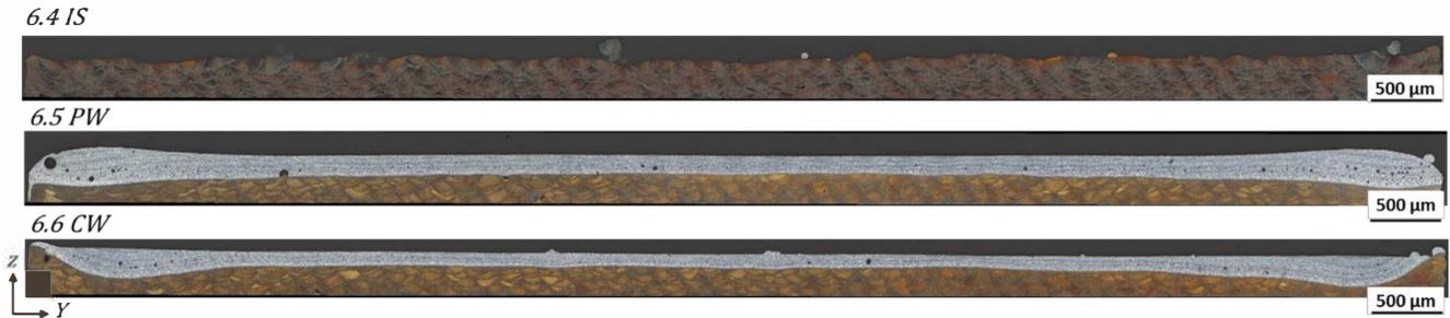
Figure 9. Etched cross sections of the cantilevers in y-direction.
