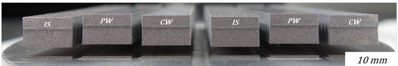
IS: initial L-PBF state, PW: polished with pulsed laser radiation, CW: polished with continuous laser radiation
