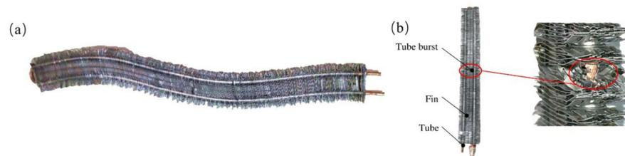
**Figure 6.** (a) Bending failure and (b) bursting failure in the sample due to hydraulic expansion.
