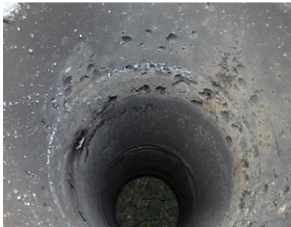
**Figure 8.** Internal localized corrosion defects in a pipeline that transports oilfield-produced water.
