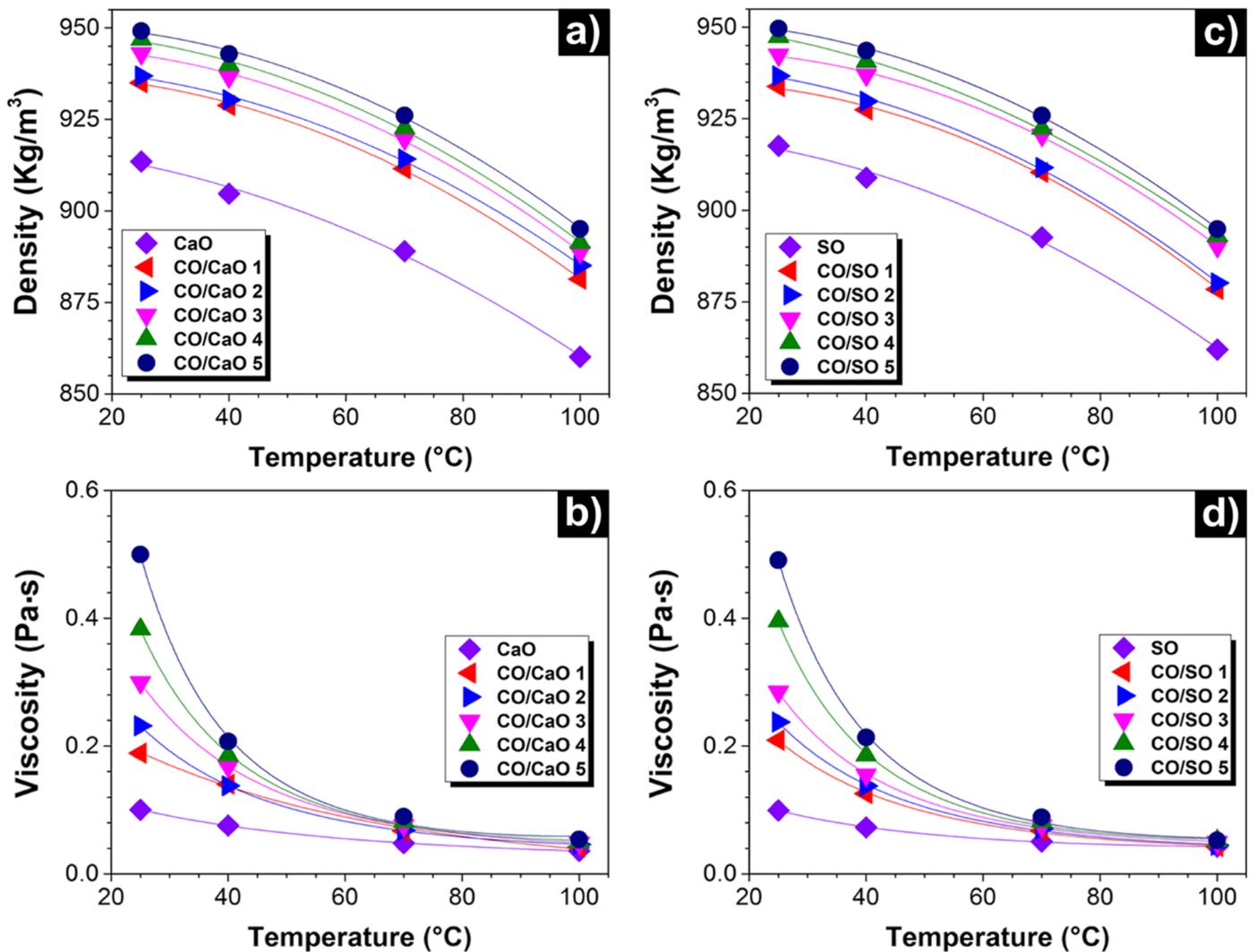
**Figure 3.** Density and dynamic viscosity of binary oil mixtures as a function of temperature: CO/CaO (a,b) and CO/SO (c,d).
