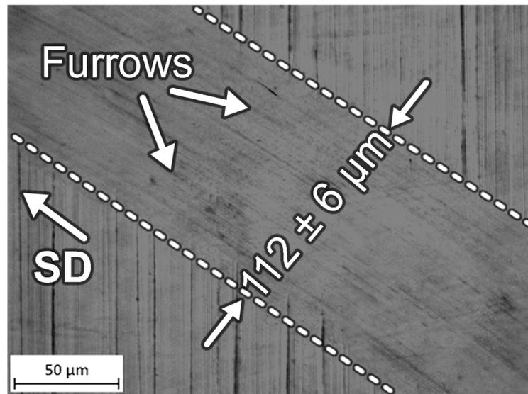
**Figure A3.** Optical micrograph of worn surface of the AISI 8620 ball tested with mineral oil.
