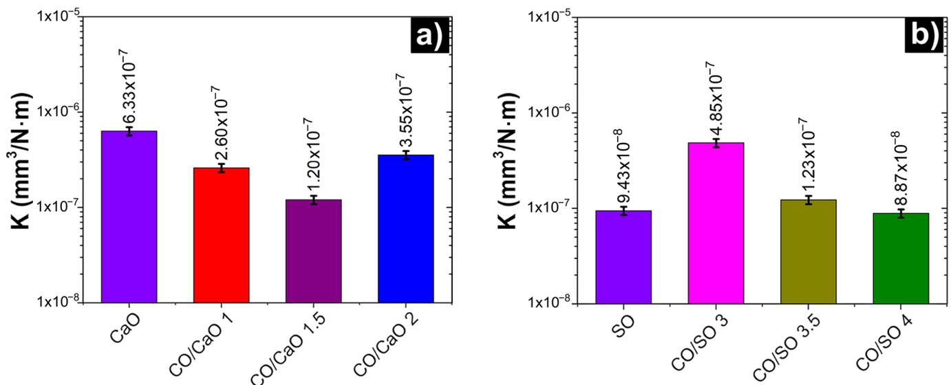
Figure 8. Influence of CO/CaO (a) and CO/SO (b) binary oil mixtures as green lubricants in the wear rate ( $K$ ) of the AISI 8620 steel.
