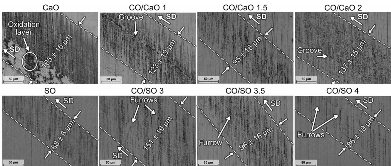
**Figure 6.** Worn surface analysis of AISI 8620 steel lubricated with canola oil, sesame oil, and their binary oil mixtures. Optical micrographs were taken at 500X. SD represents the direction of sliding.
