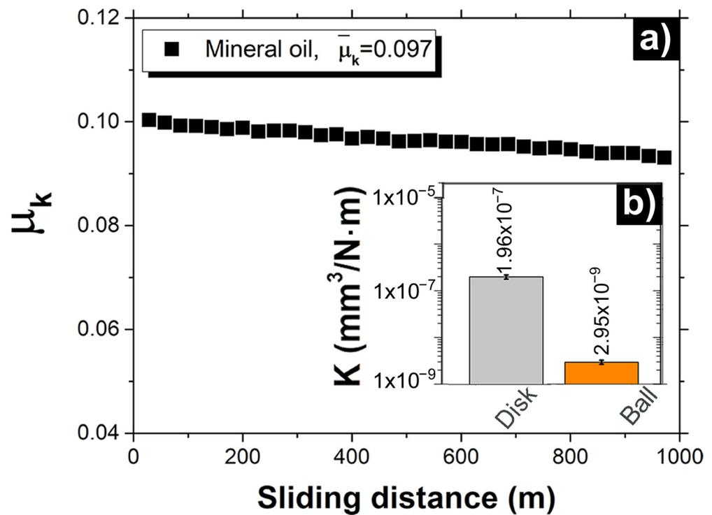
**Figure A1.** Influence of mineral oil lubricant on the kinetic friction coefficient (a) and wear rate (b) of the ISO 100Cr6/AISI 8620 steel bearing system.
