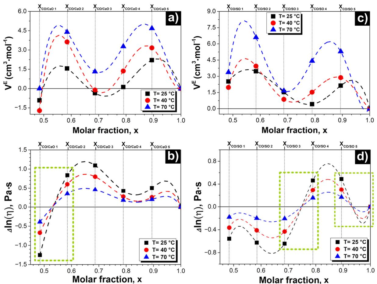
**Figure 4.** Excess molar volume ( $V^E$ ) and viscosity deviation ( $\Delta \ln(\eta)$ ) of binary mixtures at different temperatures: CO/CaO (a,b) and CO/SO (c,d).
