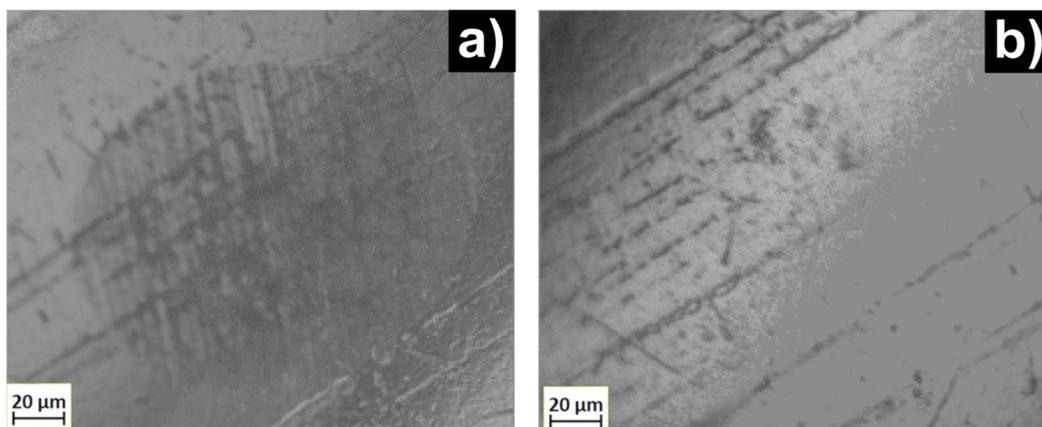
**Figure A2.** Optical micrographs of worn surfaces of the ISO 100Cr6 ball tested with the mineral oil (a) and a natural lubricant (CO/SO 4) (b).
