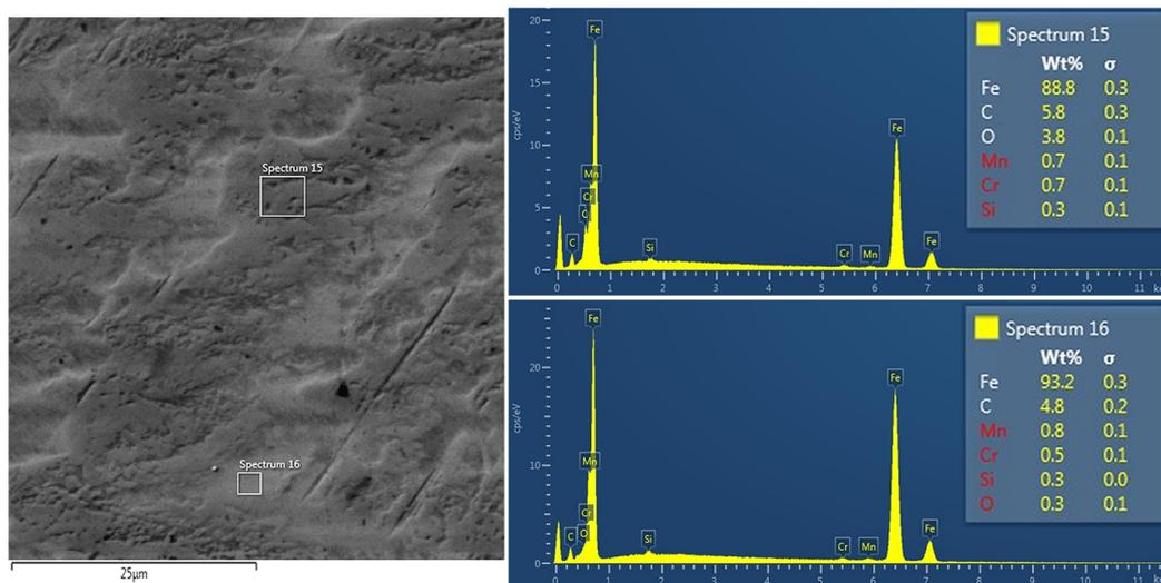
Figure 7. SEM and EDS analysis on the worn surface of AISI 8620 steel lubricated with canola oil.
