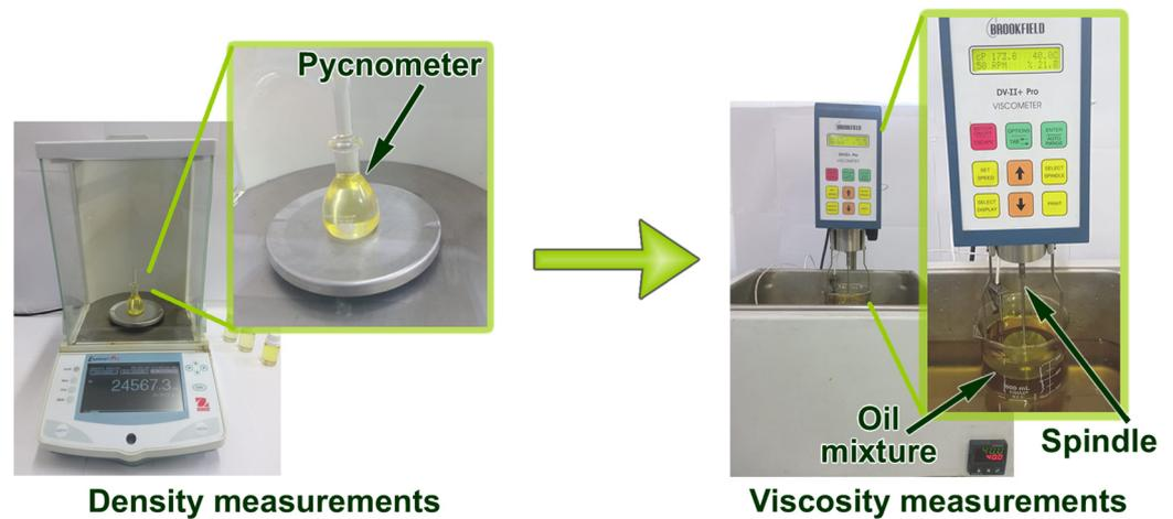
**Figure 1.** Configuration for physical characterization of binary oil mixtures.
