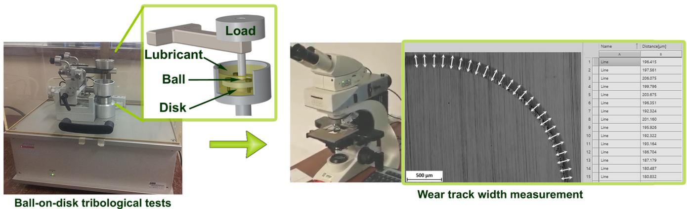
Figure 2. Configuration for friction studies and wear measurements.
