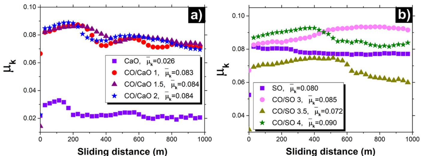
**Figure 5.** Influence of CO/CaO (a) and CO/SO (b) binary oil mixtures as green lubricants in the kinetic friction coefficient ( $\mu_k$ ) of the 100Cr6/8620 steel system.
