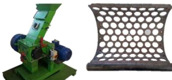
**Figure 4.** Universal granulator UG 300 (left), and outlet grate (right).
