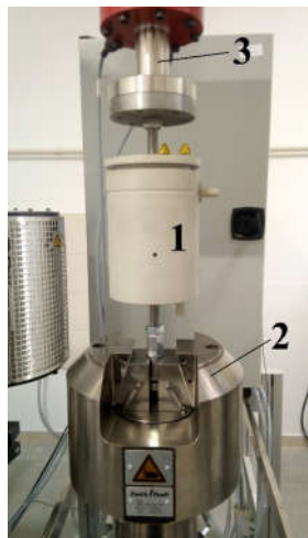
Figure 3. View of the electrochemical charging cell mounted in the mechanical testing machine: (1) cell; (2) moving jaw; (3) load cell connected to stationary beam.
