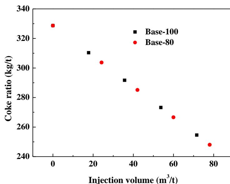
**Figure 11.** Coke ratio of blast furnace under different suitable gas injection volumes.
