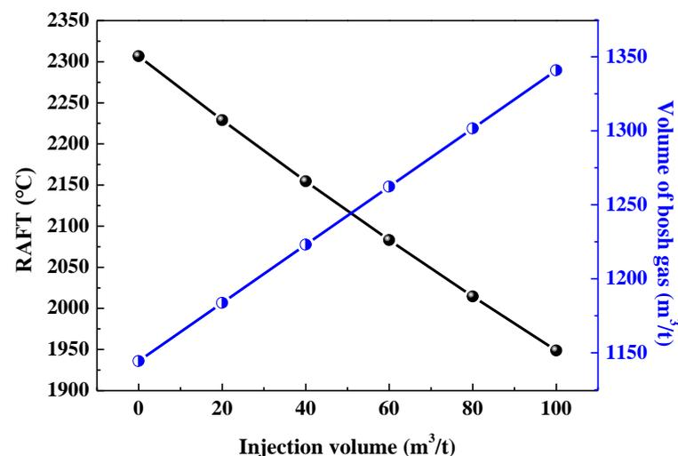
**Figure 3.** Effect of NG injection on the RAFT and volume of bosh gas.
