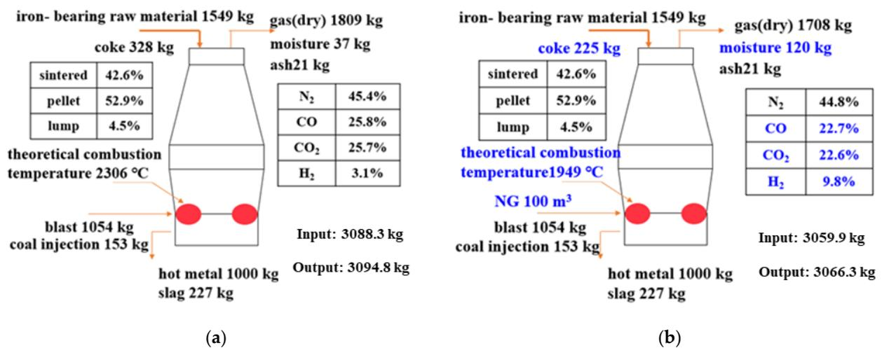
**Figure 1.** Comparison of mass flow for base case (a), and injection of 100 m<sup>3</sup>/t NG without thermal compensation (b).
