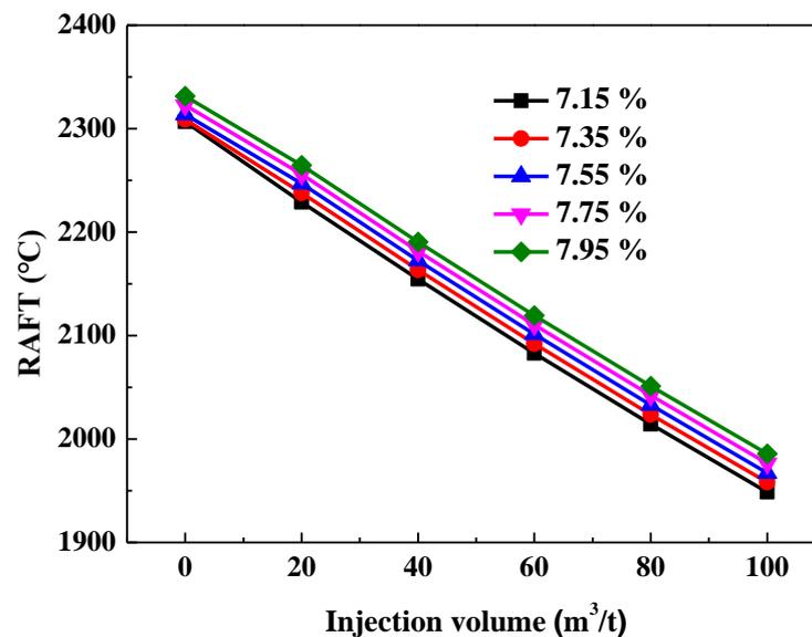
Figure 12. Effect of NG injection on RAFT under different oxygen enrichment rates.
