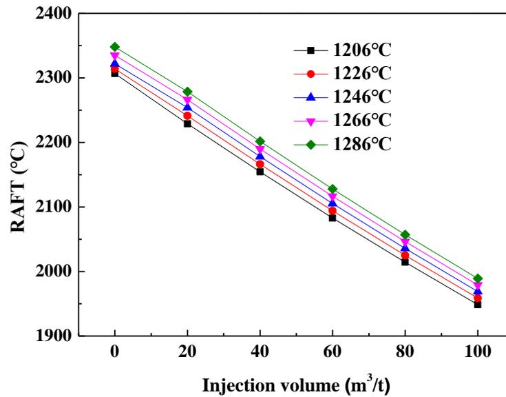
Figure 9. Effect of NG injection on RAFT under different blast temperatures.
