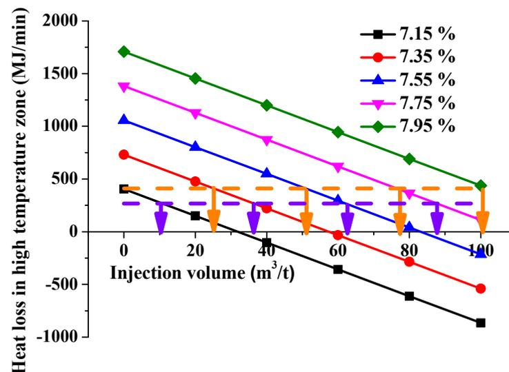
Figure 13. Effect of NG injection on heat loss in the high temperature zone of blast furnace under different oxygen enrichment rates.
