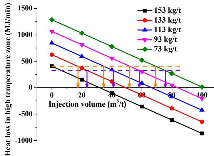
Figure 5. Effect of NG injection on heat loss in the high temperature zone of blast furnace under different coal ratios.
