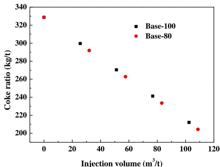
**Figure 14.** Effect of acceptable quantities of NG on the coke ratio under different oxygen enrichment rates.
