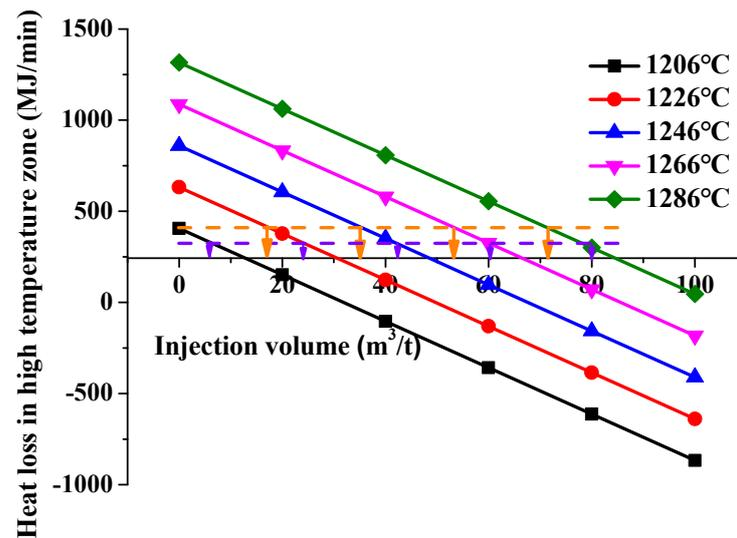
Figure 10. Effect of NG injection on heat loss in the high temperature zone of blast furnace under different blast temperatures.
