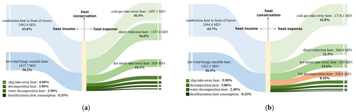
**Figure 2.** Heat balance in the high temperature zone for base case (a) and injection of 100 m<sup>3</sup>/t NG conditions without thermal compensation (b).
