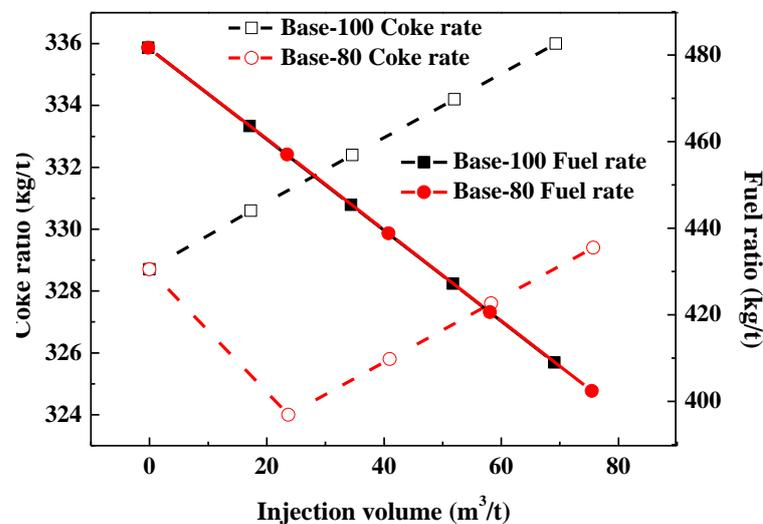
Figure 8. Coke ratio and fuel ratio of the blast furnace under different suitable gas injection volumes.
