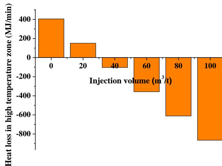
Figure 4. Effect of NG injection on heat loss in the high temperature zone.
