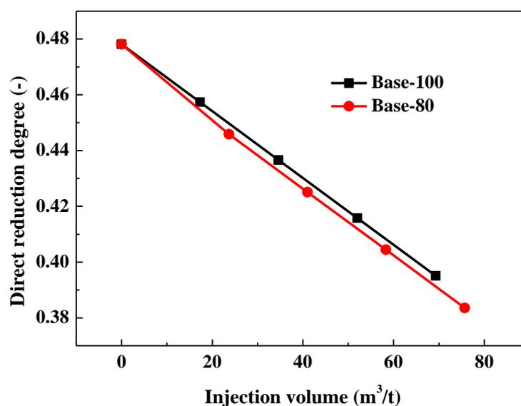
**Figure 7.** Direct reduction degrees of blast furnace under different suitable gas injection volumes.
