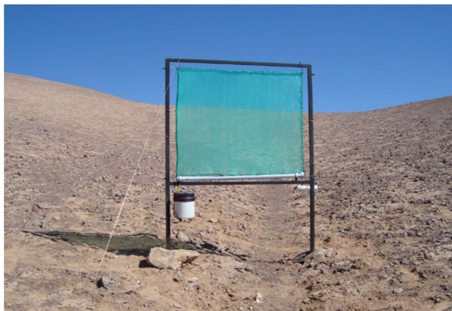
Figure 2. Fog water collector positioned nearby the P3 site. A 1 \times 1 \text{ m}^2 polypropylene Raschel mesh was mounted in a metal frame structure. It was equipped with a T/RH Hobo logger sensor (bottom right side) and a Hobo Onset logging rain gauge model RG2-M (bottom left side).
