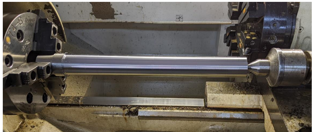
Figure 2. The workpiece geometry and the way of mounting (clamping and supporting). The dimensions shown in the figure are given in mm.
