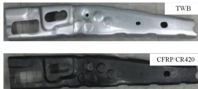
**Figure 4.** B pillars made of CFRP/CR420 composite structure and TWB. Reprinted with permission from [26]. Copyright 2017, Elsevier.
