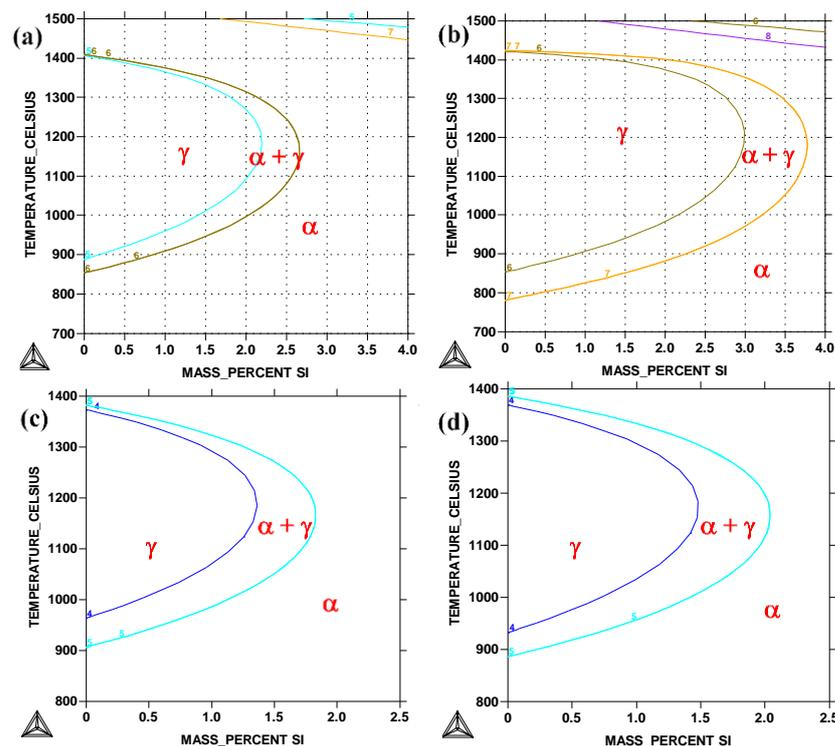
**Figure 15.** Calculated phase diagrams of different Al contents. (a) Fe-Si-0.5Mn; (b) Fe-Si-1.37Mn; (c) 1#; (d) 2#.
