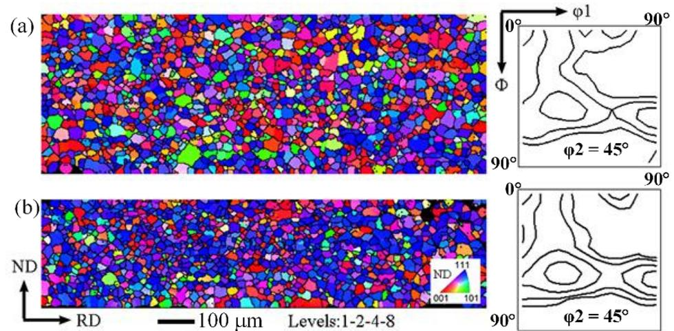
**Figure 4.** EBSD maps of recrystallized structure and textures in two sheets with different rolling reductions in 2# sample annealed at 900 °C. (a) 0.5 mm; (b) 0.35 mm.
