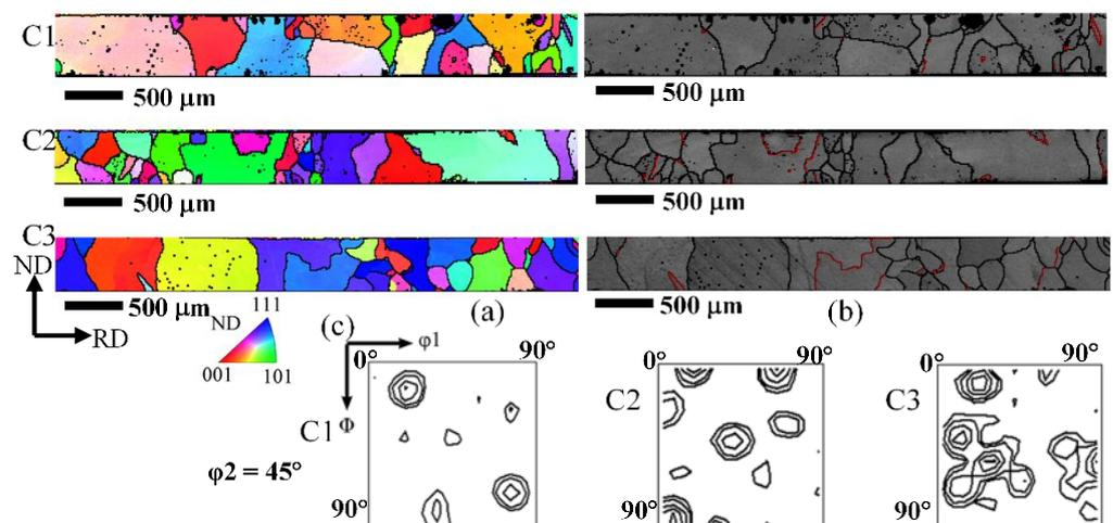
**Figure 11.** EBSD maps of 1# sheets after final transformation treatment by heating to 1150 °C under three conditions C1 to C3 following cold rolling of hot bands to 0.5 mm. (a) IPF-ND maps; (b) band contrast maps (red lines:  $\Sigma 3$ ); (c) ODFs at  $\phi_2 = 45^\circ$  section.
