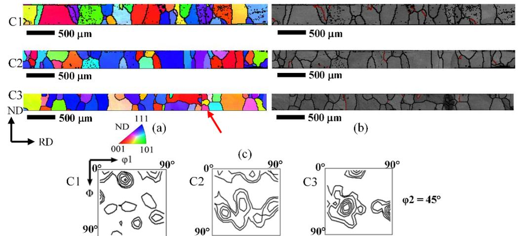
**Figure 14.** EBSD maps of 2# sheets after final transformation treatment under three conditions C1 to C3 of cold rolled 0.35 mm sheets from hot-rolled bands. (a) IPF-ND maps; (b) band contrast maps (red lines:  $\Sigma 3$ ); (c) ODFs at  $\phi_2 = 45^\circ$  section. Red arrow in (a) indicates a small region of two-layer grains in C3-processed sheet.
