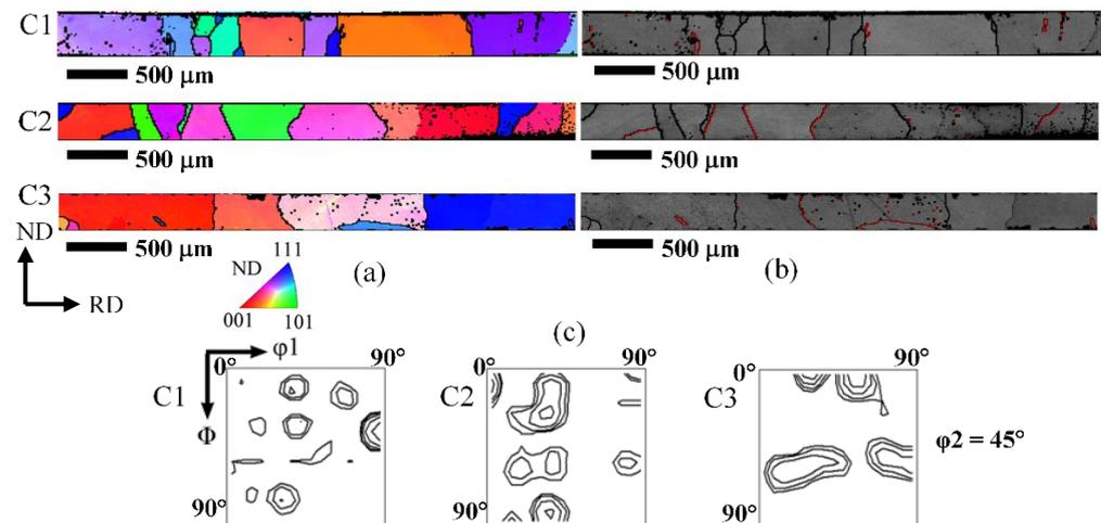
**Figure 12.** EBSD maps of 1# sheets after final transformation treatment under three conditions C1 to C3 of cold rolled 0.35 mm sheets from initial hot-rolled plates. (a) IPF-ND maps; (b) band contrast maps (red lines:  $\Sigma 3$ ); (c) ODFs at  $\phi_2 = 45^\circ$  section.
