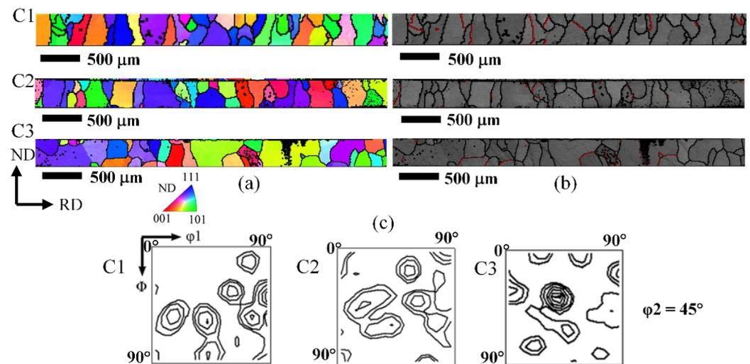
**Figure 10.** EBSD maps of 2# sheets after final transformation treatment by 1150 °C of three conditions C1 to C3 following cold rolling of columnar grained samples to 0.35 mm. (a) IPF-ND maps (b) band contrast maps with boundary characters (red lines:  $\Sigma 3$ ); (c) ODFs at  $\phi_2 = 45^\circ$  section.
