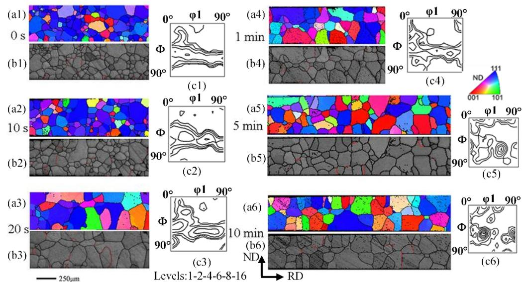
**Figure 6.** The microstructure and texture evolution during transformation treatment in 2# sheets at different holding times. Starting from hot-rolled sheets, cold rolling to 0.5 mm with 80% reduction. Heating to 1050 °C for different time and cooled either by water quenching (a1–a3) or 5 °C/min in  $H_2$  of 4 L/min (a4–a6). (a1–a6) IPF-ND maps, (b1–b6) band contrast maps (red lines:  $\Sigma 3$  boundary) and (c1–c6) ODFs at  $\phi_2 = 45^\circ$  section.
