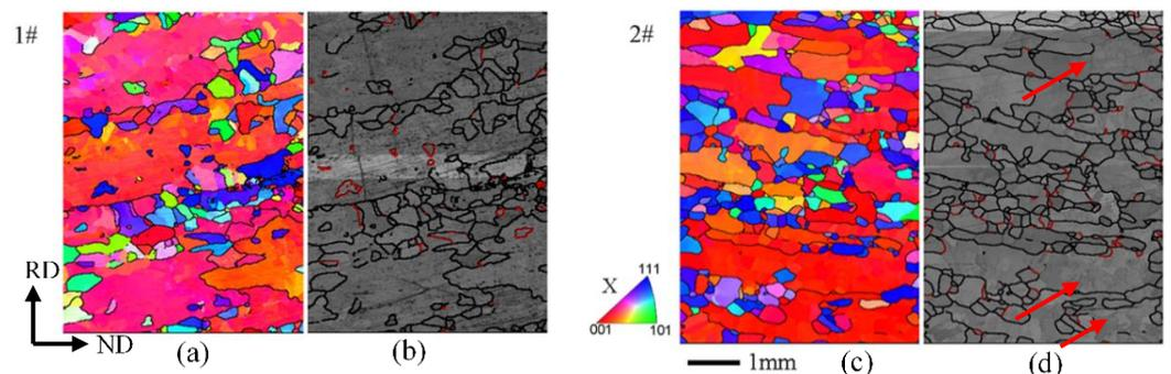
**Figure 2.** EBSD maps of 1# (1%Si) and 2# (0.72%Si) cast slabs. (a,c) IPF-ND map and (b,d) band contrast maps with grain boundaries characters (red:  $\Sigma 3$ ).
