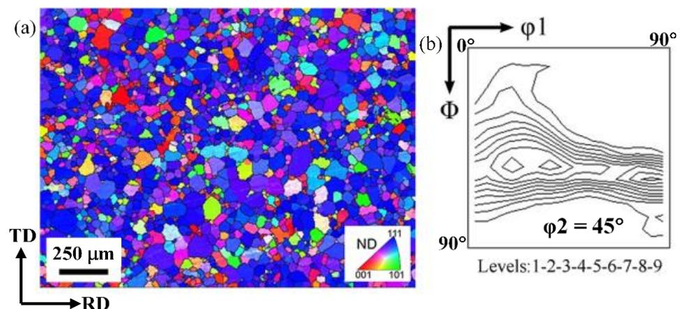
**Figure 5.** EBSD map of commercial 800-grade electrical steel measured on rolling plane. (a) orientation map; (b) orientation distribution function (ODF) figure at  $\phi_2 = 45^\circ$  section.
