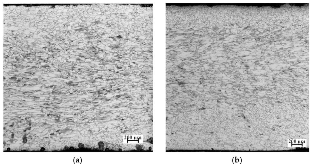
**Figure 3.** Micrographs in transverse section of hot-rolled sheets 1# (a) containing 1%Si and 2# (b) containing 0.72%Si.
