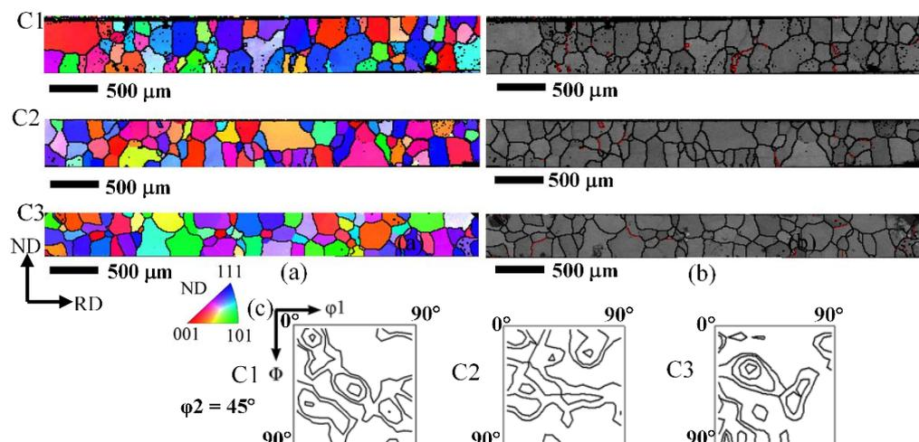
**Figure 13.** EBSD maps of 2# sheets after final transformation treatment under three conditions C1 to C3 of cold rolled 0.5 mm sheets from initial hot-rolled structure. (a) IPF-ND maps; (b) band contrast maps (red lines:  $\Sigma 3$ ); (c) ODFs at  $\phi_2 = 45^\circ$  section.
