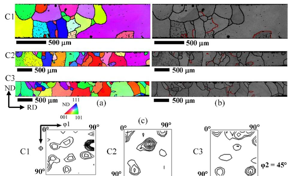
**Figure 7.** EBSD maps after final transformation treatment under 3 different processing parameters C1 to C3 of 1# sample, 0.5 mm thickness. (a) EBSD maps of IPF-ND, (b) Band contrast maps (red line:  $\Sigma 3$ ); (c) ODFs at  $\phi_2 = 45^\circ$  section.
