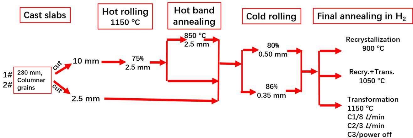
**Figure 1.** Schematic diagram of processing steps.
