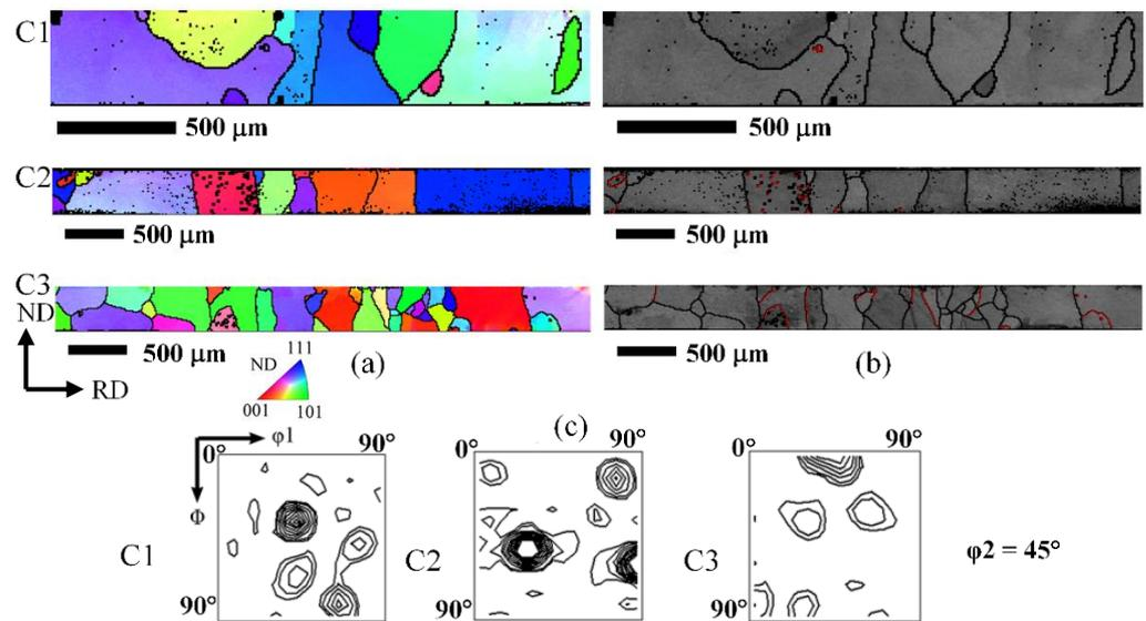
**Figure 8.** EBSD maps of 1# sheets similarly processed on 0.35 mm cold rolled sheets after final transformation treatment at 1150 °C under three conditions C1 to C3. (a) EBSD maps of IPF-ND, (b) Band contrast maps (red line:  $\Sigma 3$ ); (c) ODFs at  $\phi_2 = 45^\circ$  section.
