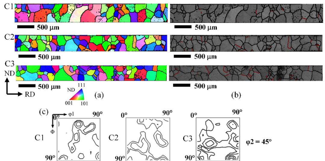
**Figure 9.** EBSD maps of 2# samples after final transformation treatment by 1150 °C of three conditions C1 to C3 on the 0.5 mm cold rolled sheets with initial columnar grain structure. (a) IPF-ND maps; (b) band contrast maps with boundary characters (red lines:  $\Sigma 3$ ); (c) ODFs at  $\phi_2 = 45^\circ$  section.
