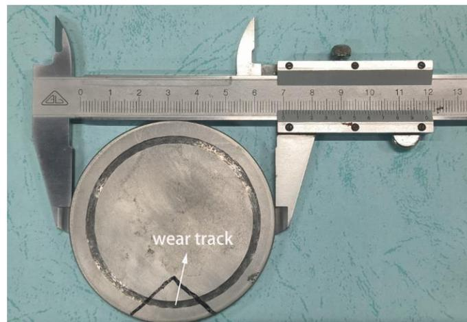
**Figure 1.** 7075-T6 aluminum alloy after tribocorrosion test.
