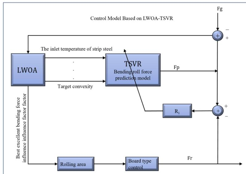
Figure 3. Static component control model based on LWOA-TSVR algorithm.
