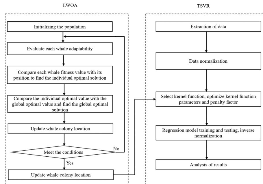
Figure 5. The process of LWOA optimized TSVR.
