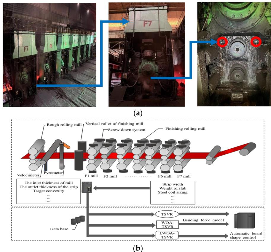
**Figure 1.** Layout of finishing the mill line: (a) Bending roll of finishing mill; (b) Equipment layout of hot continuous rolling mill line.
