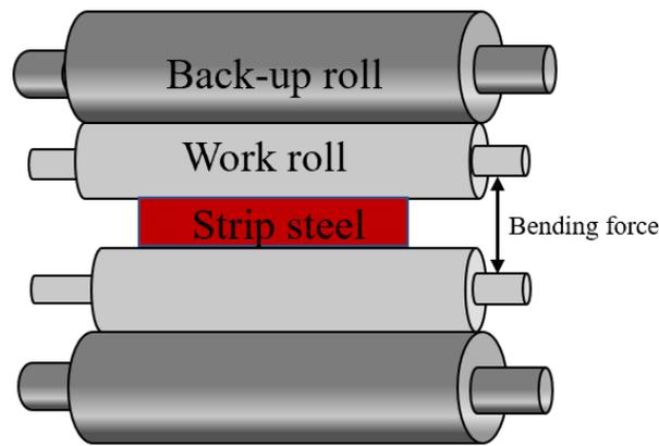
Figure 2. F7 mill hydraulic roll bending schematic.
