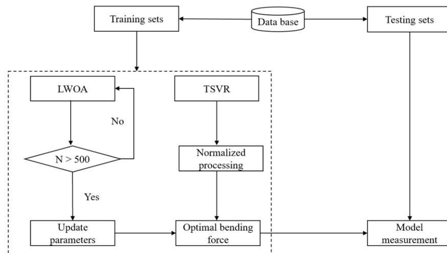
Figure 4. Flow chart of the bending force prediction model.
