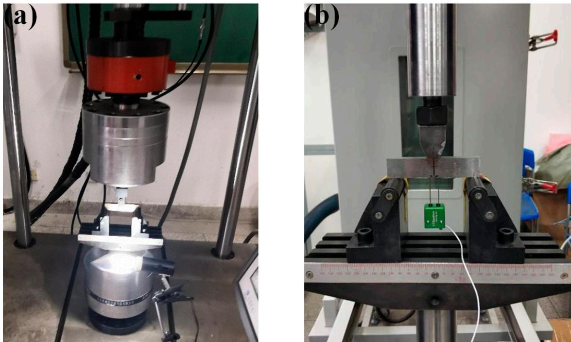
**Figure 4.** (a) Micro pre-crack (0.10 W) was prefabricated in the location of notch tip by an Electro-Hydraulic Servo Fatigue Testing Machine (SDS-300) with a 300 KN load cell; (b) three-point bending experiment was performed using an electronic universal testing machine (AGS-X) with a 100 KN load cell.
