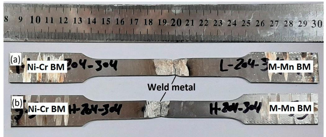
Figure 11. Photograph of the tensile specimens showing the location of fracture in the weld metals: (a) at low heat input; (b) at high heat input.
