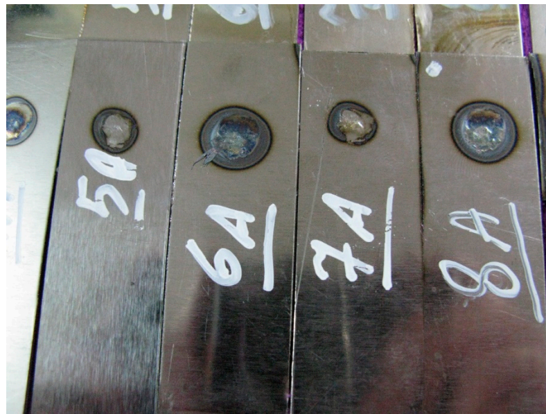
Figure 3. Some of the welded specimens by RSW according to Table 3 experiments.
