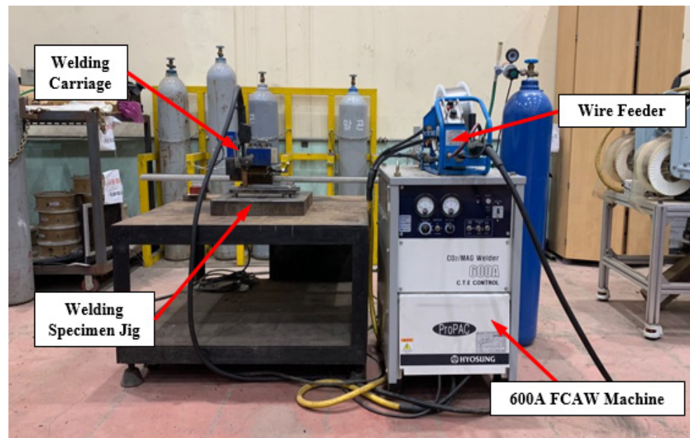
Figure 1. Experimental setup for flux cored arc welding [7].
