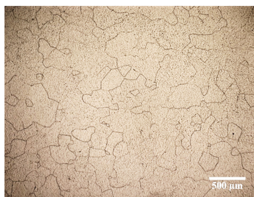
Figure 1. Microstructure of Ti55511 before deformation of a double-cone sample at 950 °C.
