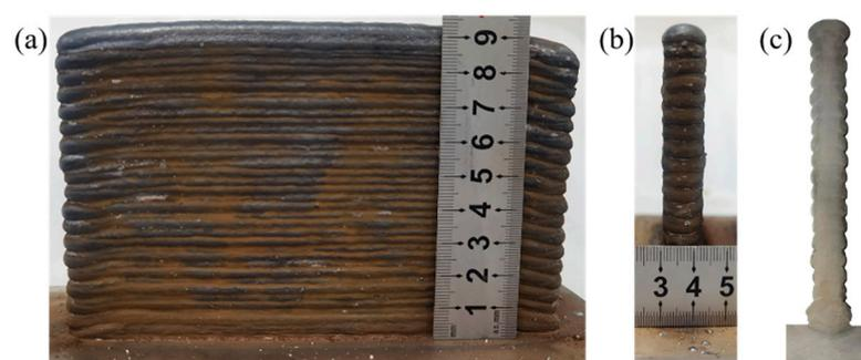
**Figure 3.** The single-layer multi-channel deposition part: (a) front; (b) flank; (c) profile.
