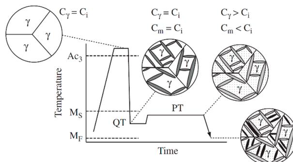
**Figure 1.** Thermal process to develop QP steels. QT and PT correspond to quenching and partitioning temperatures [5]. Copyright obtained from Elsevier.  $C_i$ ,  $C_\gamma$ , and  $C_m$  are the carbon contents of the initial alloy, austenite, and martensite, respectively. Reproduced with permission of the editor.
