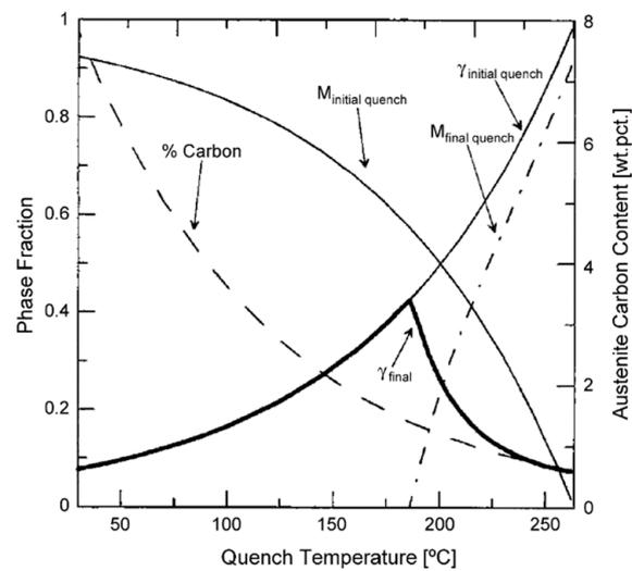
**Figure 2.** Predicted phase fractions of the microstructure after the QP process [5]. Copyright obtained from Elsevier. The solid bold line corresponds to the final austenite fraction at room temperature. Solid lines illustrate the austenite ( $\gamma$ ) and martensite (M) fraction at the first quenching temperature, and the dash-dotted line represents the as-quenched or fresh martensite that forms during the final quench. Reproduced with permission of the editor.
