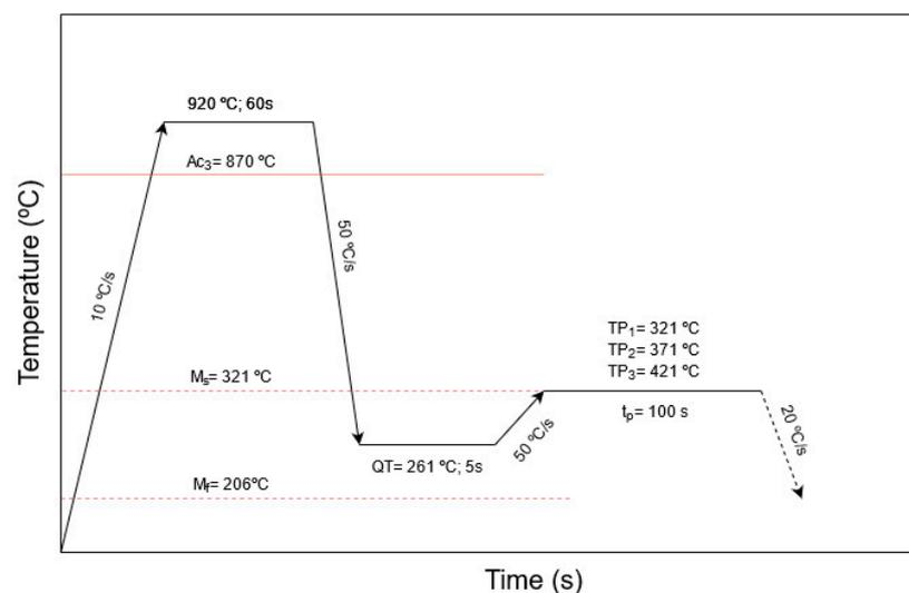
**Figure 3.** Schematic of the heat treatments applied to the present steel.
