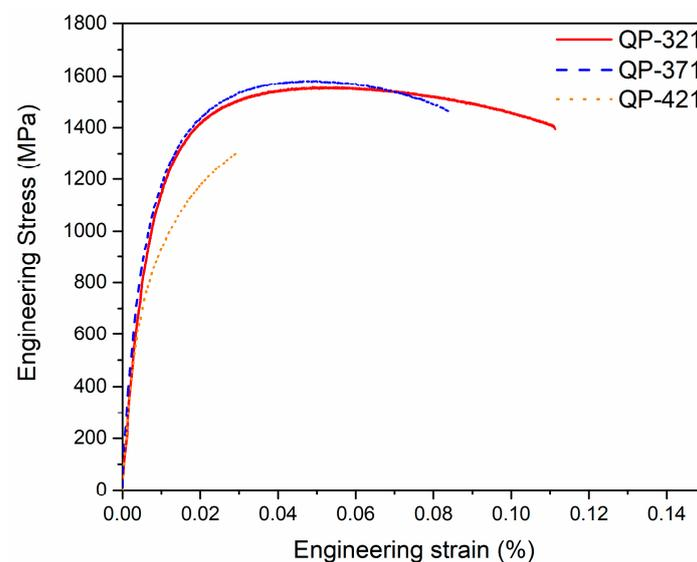
**Figure 11.** Tensile properties of the studied steel QP-x.
