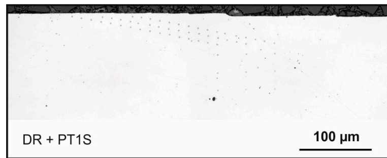
Figure 7. Example for the obliquely placed indentations to measure the hardness of the near surface area.
