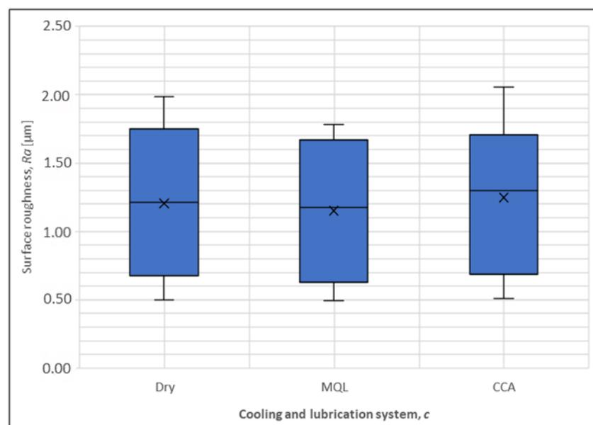
Figure 8. Surface roughness vs cooling/lubrication system, box, and whisker plot.
