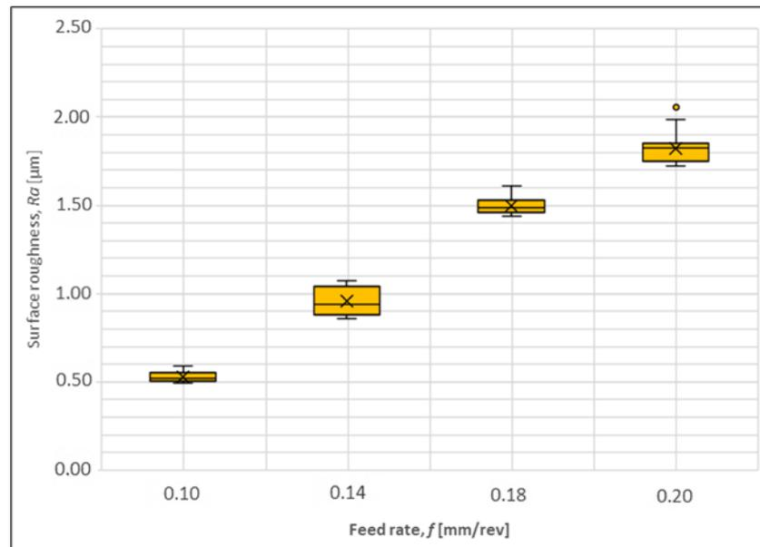
Figure 7. Surface roughness vs feed rate, box, and whisker plot.
