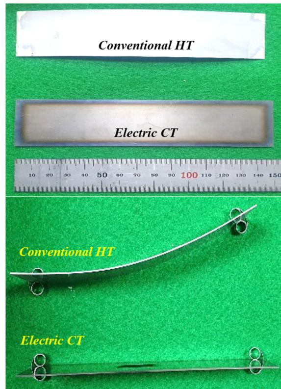
**Figure 8.** Shape changes in CP Ti sheet after applying conventional heat treatment and electric current treatment at 600 °C.
