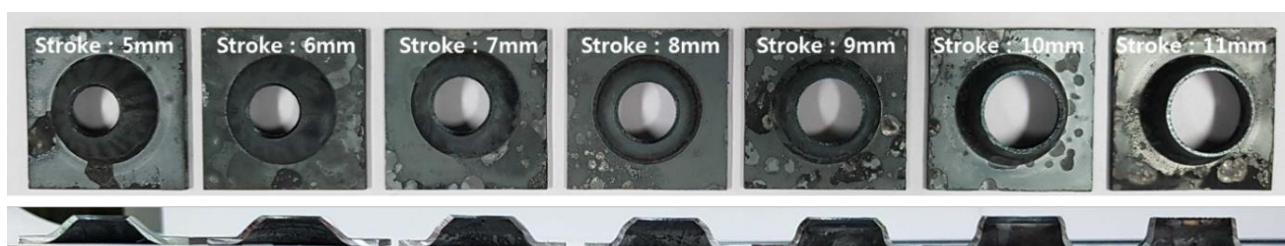
Figure 8. Extruded collar shape according to stroke.
