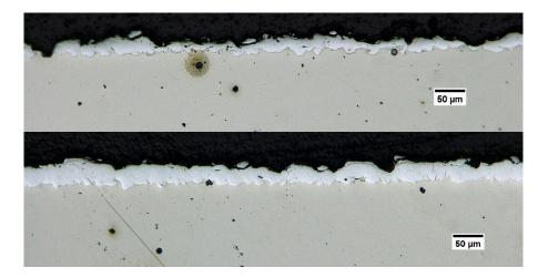
**Figure 14.** Optical micrographs showing cross sections of cold spray deposits for unprocessed Cr (top) and dried Cr (bottom).
