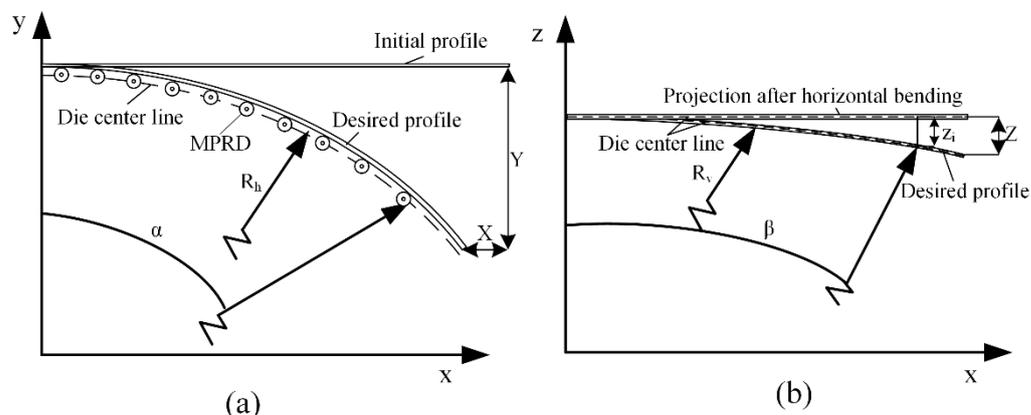
Figure 3. Trajectory design of clamp and MPRD. (a) Horizontal bending. (b) Vertical bending.
