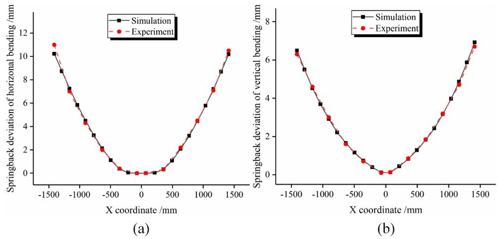
Figure 14. Comparison of springback deviation of Y-profile: (a) horizontal bending, (b) vertical bending.
