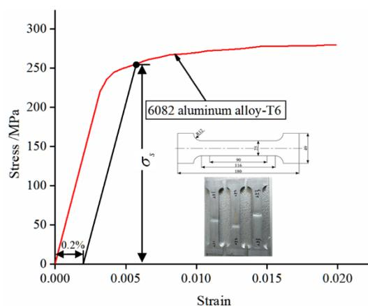
**Figure 1.** Stress–strain curve of 6082 aluminum alloy.
