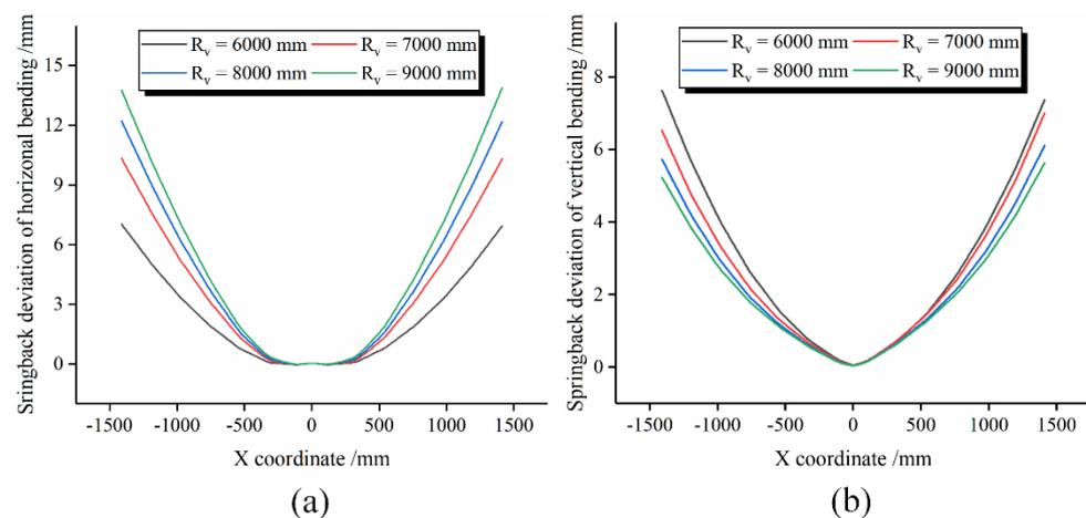
**Figure 7.** Springback deviation with different vertical bending radii. (a) Springback deviation of horizontal bending. (b) Springback deviation of vertical bending.
