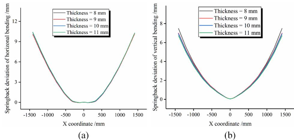
**Figure 11.** Springback deviation with different wall thickness of the profile. (a) Springback deviation of horizontal bending. (b) Springback deviation of vertical bending.
