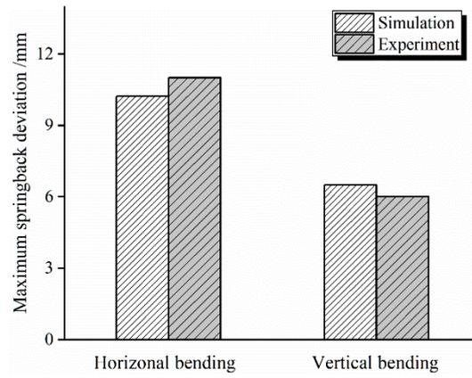
Figure 15. Comparison of maximum springback deviation.
