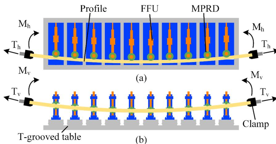
**Figure 2.** Forming principle of FSB-MPRD. (a) Horizontal bending process. (b) Vertical bending process.
