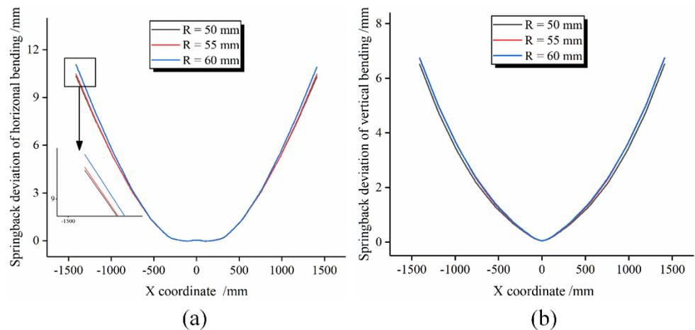
**Figure 10.** Springback deviation with different radii of roller dies. (a) Springback deviation of horizontal bending. (b) Springback deviation of vertical bending.
