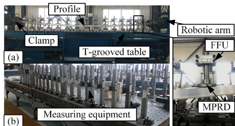
**Figure 12.** Experimental equipment. (a) FSB-MPRD experimental equipment. (b) Measuring equipment.
