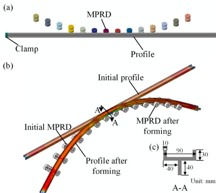
**Figure 4.** Finite element model. (a) Diagram of model assembly. (b) Numerical simulation results. (c) Cross-section of the Y-profile.
