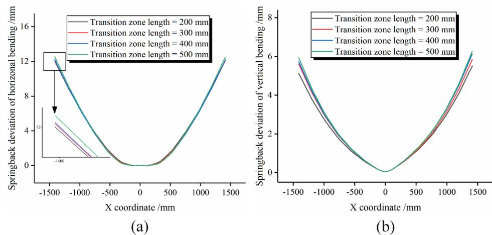
**Figure 9.** Springback deviation with different transition zone lengths. (a) Springback deviation of horizontal bending. (b) Springback deviation of vertical bending.
