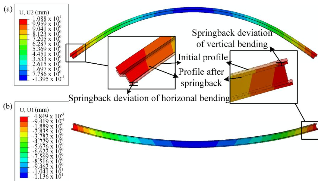
**Figure 5.** Characterization of springback. (a) Definition of springback deviation of horizontal bending. (b) Definition of springback deviation of vertical bending.
