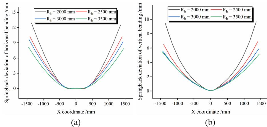
**Figure 6.** Springback deviation with different horizontal bending radii. (a) Springback deviation of horizontal bending. (b) Springback deviation of vertical bending.
