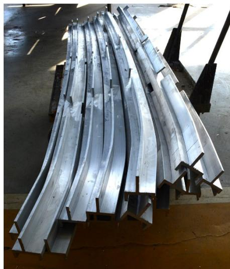
Figure 16. Large-scale production of the Y-profile.
