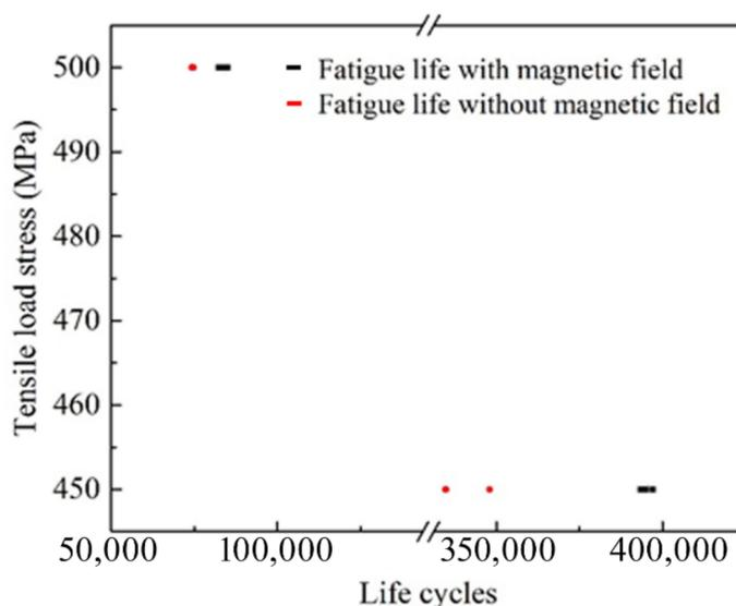
Figure 2. The fatigue life cycle under the load of 450 MPa and 500 MPa, with and without magnetic field.
