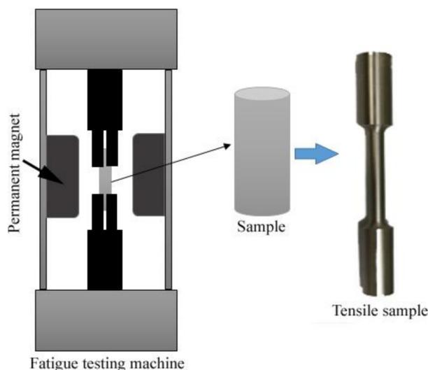
**Figure 1.** The illustration of fatigue tests containing magnetic field and the corresponding samples.
