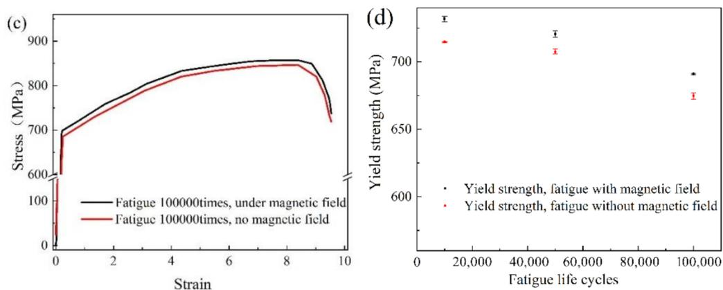
**Figure 3.** The stress–strain curves of specimens after fatigue life of 10,000 cycles (a), 50,000 cycles (b), 100,000 cycles (c), and yield strength conducted by different fatigue tests life cycles (d) under the load of 450 MPa.
