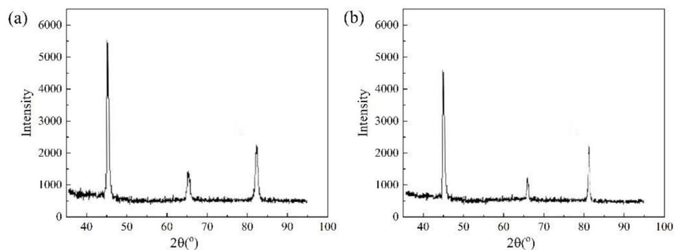
**Figure 5.** The X-ray diffraction patterns of the specimen that experienced fatigue tests of 450 MPa for 10,000 cycles under magnetic field of 1.2–1.3 T (a) or no magnetic field (b).
