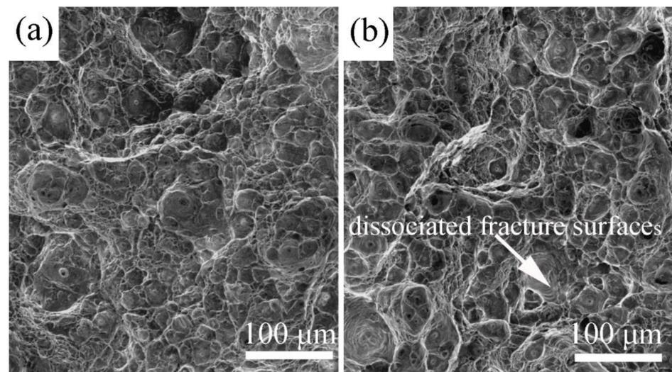
**Figure 6.** The SEM photographs of fracture morphology of tensile specimens that experienced fatigue tests of 50,000 cycles under the load of 450 MPa, (a) with magnetic field and (b) without magnetic field.
