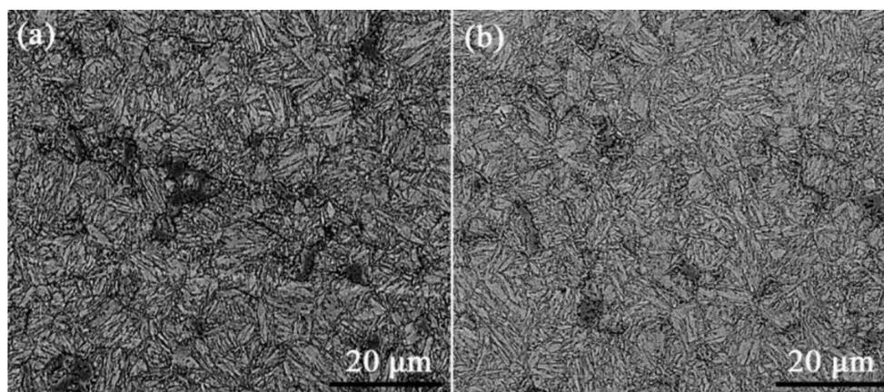
**Figure 4.** The SEM photographs of the specimen that experienced fatigue tests of 450 MPa for 10,000 cycles under magnetic field of 1.2–1.3 T (a) and no magnetic field (b).
