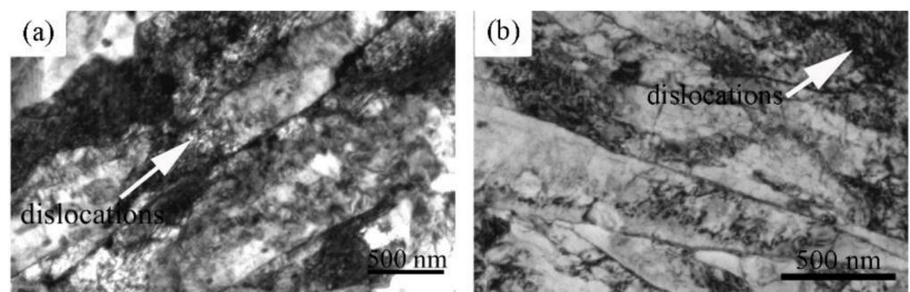
**Figure 7.** The TEM photographs of the specimen that experienced fatigue tests of 450 MPa for 10,000 cycles under magnetic field (a) and no magnetic field (b) of 1.2–1.3 T, revealing obvious dislocation tangles.
