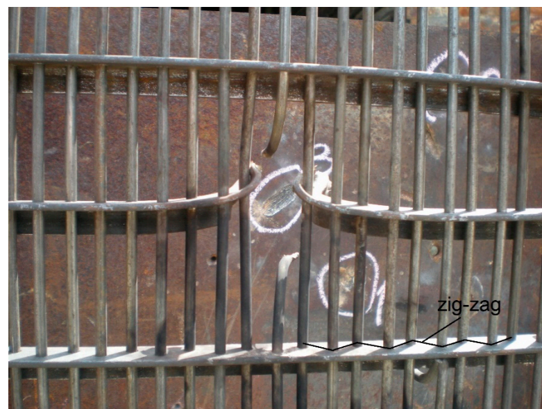
Figure 2. Patented wires in a zig-zagged configuration useful in causing projectile yaw. Zig-zag configuration of patented wires is indicated by a broken black line [15].
