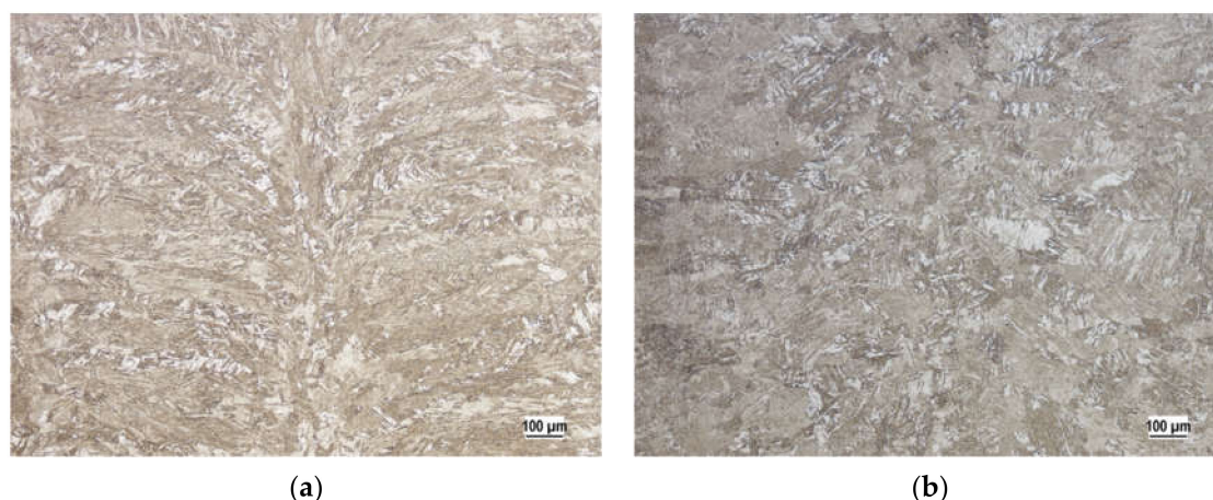
Figure 9. (a) The microstructure of the welded metal of the electron beam for the high-strength steel S960 QL. (b) The microstructure of the welded metal of the laser beam for the high-strength steel S960 QL.
