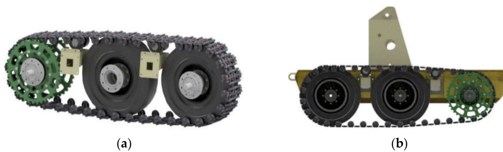
Figure 2. (a) A drive-system of the demining machine Božena 5; (b) a side-view of a model.
