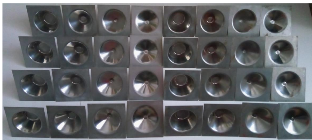
Figure 16. Parts machined according to array of experiments, reprinted with permission from ref. [5].
