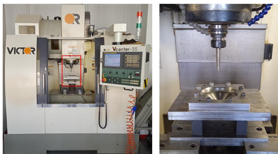
Figure 9. Technological setup used for the implementation of the SPIF process, adapted with permission from ref. [5].
