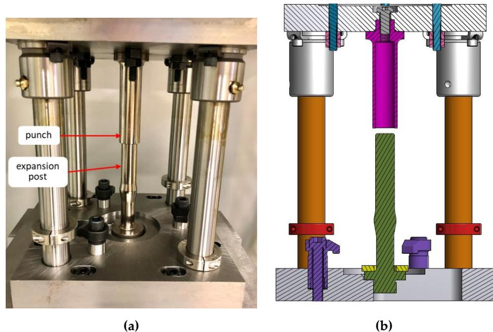
**Figure 4.** (a) Experimental setup of expansion process. Omitted is the hydraulic press. (b) Section view of expansion setup. Expansion setup uses the same die set as the extrusion process.
