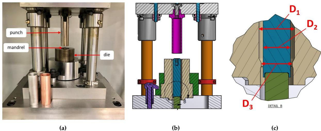
**Figure 3.** (a) Experimental setup of extrusion process which provides 52% radial strain. Omitted is the hydraulic press. Also depicted is annealed copper and aluminum test metals ready for extrusion. For size perspective, the test metals are 89 mm in height. This setup is identical to the process which enacts 68% radial strain except for dimension L. (b) Section view of extrusion setup. (c) Die cavity and extrusion ledge. The tubular bimetal is omitted.
