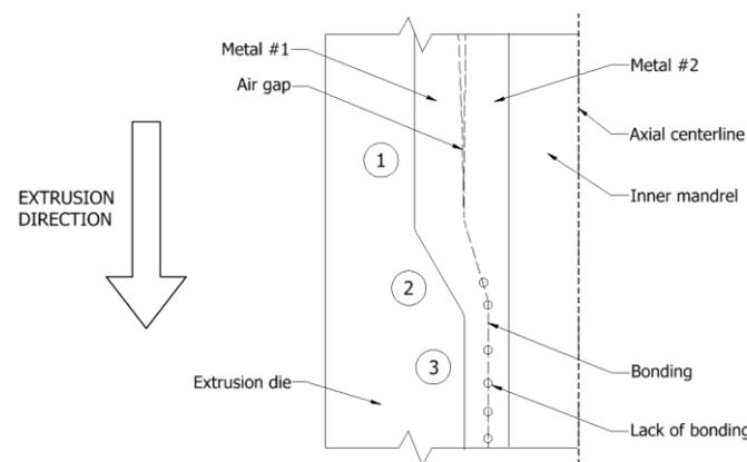
**Figure 1.** Axis-symmetric cross section of extrusion process and the three stages of bonding using AEB. The metal initially experiences compression (stage 1) before entering the extrusion zone (stage 2), where severe plastic deformation occurs, and exits in the final desired shape (stage 3).
