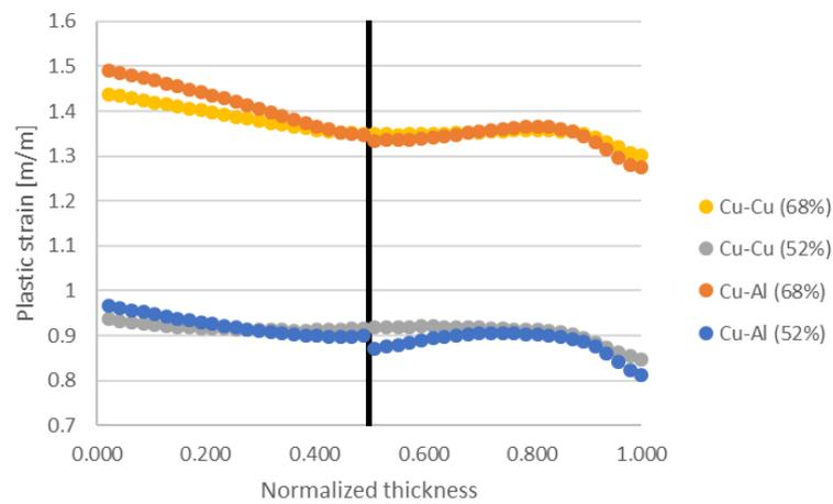
**Figure 11.** Equivalent plastic strain through the extruded wall where normalized 0.0 is the inner edge of the tubular wall and normalized 1.00 is the outer surface of the tube. Vertical line represents bonding interface location. Plastic strain is taken at the vertical midpoint of the extruded bimetal.
