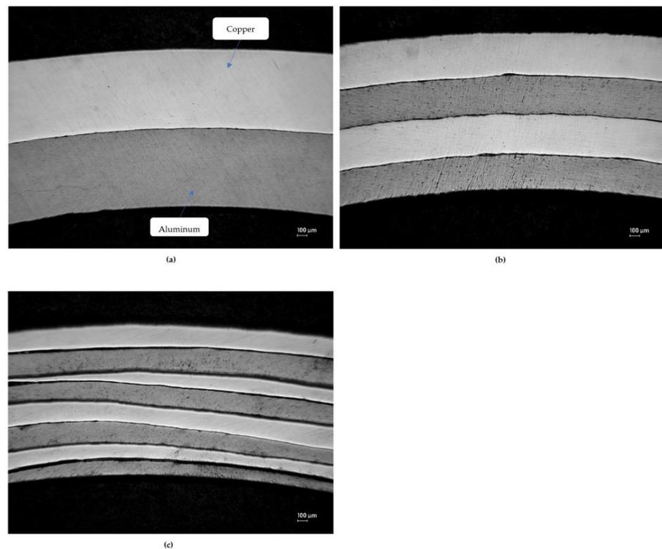
**Figure 12.** Bimetallic tube of (a) 2-layer, (b) 4-layer, and (c) 8-layer copper-aluminum, shown in the extrusion direction, produced at 52% deformation.
