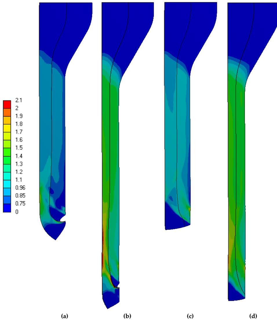
**Figure 10.** Total equivalent plastic strain at 7.62 mm of displacement for copper-aluminum at (a) 52%, and (b) 68% deformation and copper-copper at (c) 52%, and (d) 68% deformation. The die and mandrel are omitted. Units of strain are mm/mm.
