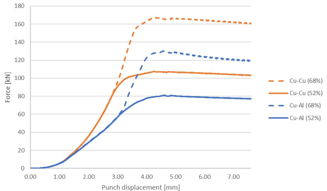
**Figure 9.** Force-displacement curve for extrusion at 52% and 68% deformation for copper-copper and copper-aluminum bimetals.
