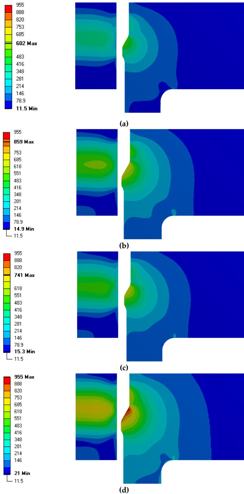
**Figure 8.** Von Mises stress within the die and mandrel during extrusion of copper-aluminum at (a) 52%, and (b) 68% deformation and copper-copper at (c) 52%, and (d) 68% deformation. The metals that experienced extrusion are omitted. Units of stress are MPa.
