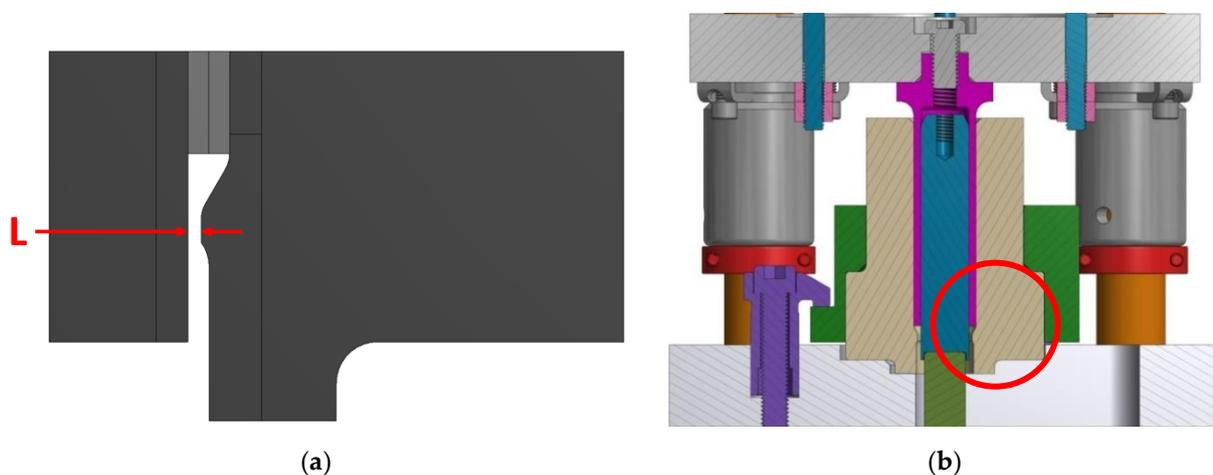
**Figure 6.** (a) Finite element geometry which represents the two deformation cases studied: 52% and 68%. Dimension L was adjusted to obtain the two different cases. (b) The experimental setup is shown at dead-bottom position, where the simulated area is identified by a red circle.
