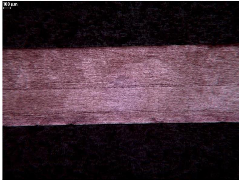
**Figure 13.** Bimetallic tube of 2-layer copper-copper, shown in the transverse direction, produced at 68% deformation.
