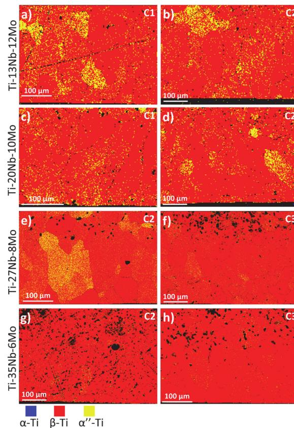
**Figure 6.** Phases obtained for the samples with surface Ti-Nb-Mo fusion: (a,b) Ti-13Nb-12Mo alloys treated under conditions C1 and C2; (c,d) Ti-20Nb-10Mo alloys treated under conditions C1 and C2; (e,f) Ti-27Nb-8Mo alloys treated under conditions C2 and C3; (g,h) Ti-35Nb-6Mo alloys treated under conditions C2 and C3. The blue phase is hexagonal Ti, the red phase corresponds to cubic Ti and the yellow phase to the orthorhombic Ti of the martensitic phase.
