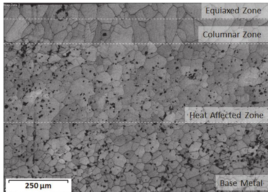
**Figure 15.** Band contrast image for the cross-section of the Ti-27Nb-8Mo alloy condition 2 and the different marked microstructural zones.
