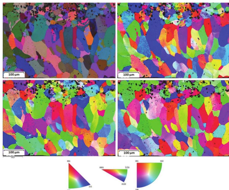
**Figure 7.** Sample Ti-27Nb-8Mo (C3). Euler color map accompanied by the inverse pole figures (IPF) diagrams in the X, Y, and Z directions. Grains are elongated in the direction of the thermal gradients, and size is determined by the base material (epitaxial growth). The grains with higher Nb contents are smaller, as Figure 7 depicts.
