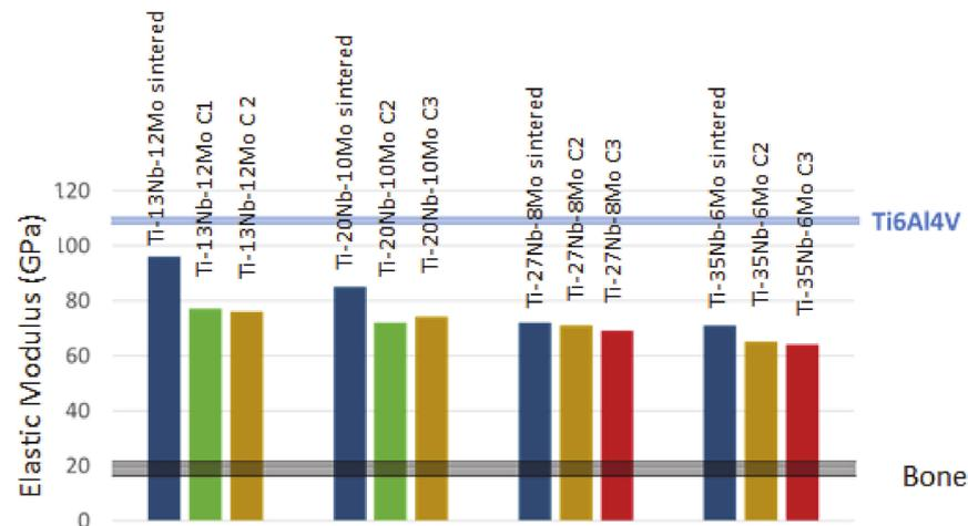
**Figure 14.** The obtained elastic modulus compared to values of bone and Ti6Al4V values.
