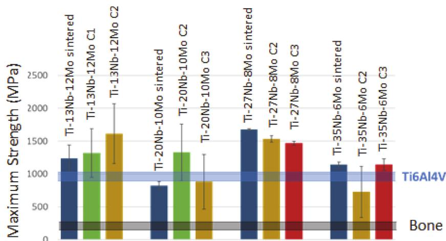
**Figure 13.** The obtained maximum resistance values compared to the values of bone and Ti6Al4V.
