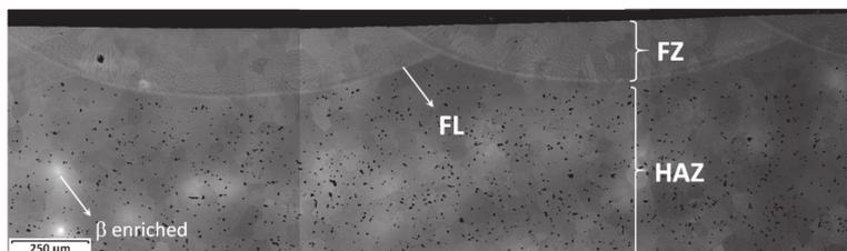
**Figure 2.** Microstructure of the Ti-13Nb-12Mo alloy treated by laser fusion under condition C1. In detail, the fusion line (FL), heat-affected zone (HAZ), and fusion zone (FZ) regions are observed.
