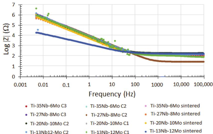
Figure 10. Bode diagrams of the all Ti-Nb-Mo samples.
