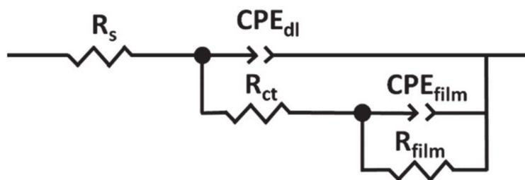
Figure 11. The electrical circuit that simulates a parallel equivalent circuit to represent a porous oxide layer, where  $R_s$  is the resistance of the solution,  $CPE_{dl}$  and  $R_{ct}$  are the constant phase element and the resistance to charge transfer, and  $CPE_{film}$  and  $R_{film}$  are the constant phase element and the resistance of the passive layer.
