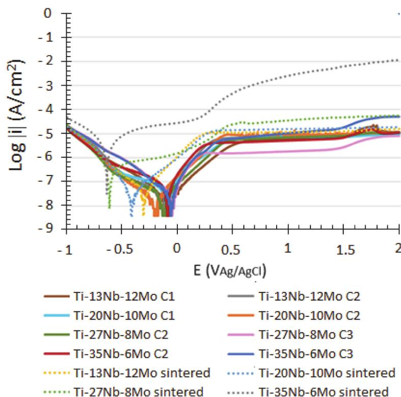
Figure 9. Potentiodynamic curves of the studied Ti-Nb-Mo alloys.
