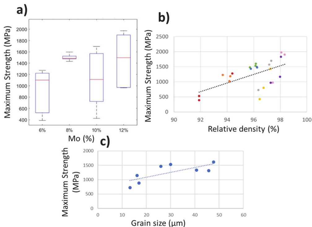
**Figure 12.** Representations of the maximum resistance obtained in the three-point bending tests: (a) Boxplots shown in accordance with the alloy’s Mo content (b,c) two scatter plots according to relative density and grain size.
