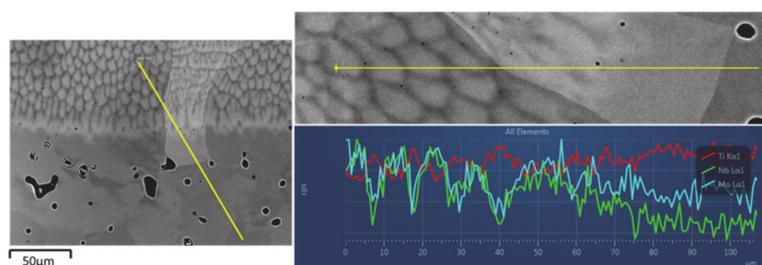
**Figure 4.** Line Energy-dispersive X-ray spectroscopy (EDS) analysis of the Ti-20Nb-10Mo alloy microstructure (C1).
