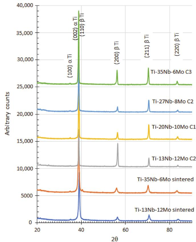
**Figure 1.** Diffraction patterns of the samples under the different laser treatment conditions and sintered.
