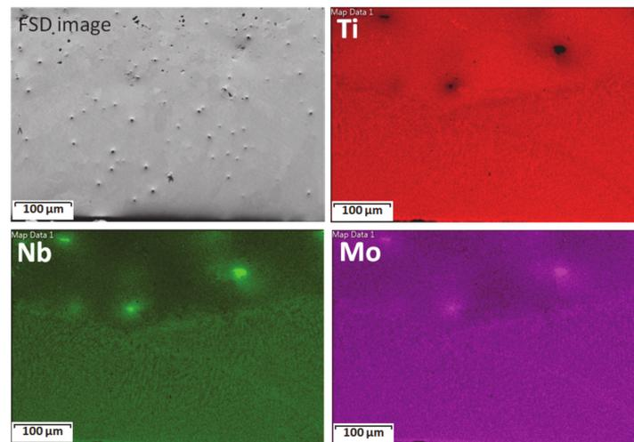
**Figure 5.** Map of the distribution of Ti, Nb, and Mo of the Ti-27Nb-8Mo alloy in its C3, using Forward Scatter Detector (FSD).
