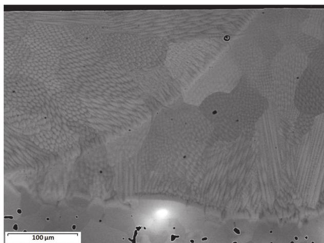
**Figure 3.** Detail of the FZ microstructure in the Ti-20Nb-10Mo alloy (C2).
