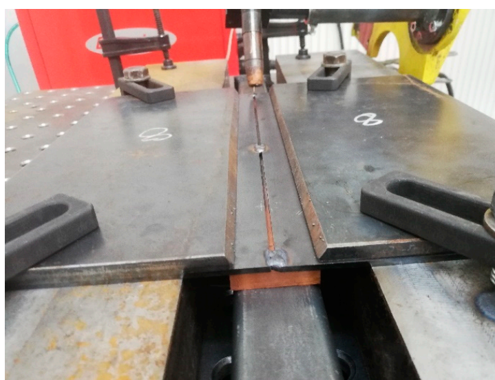
Figure 2. Welding with accelerated cooling.
