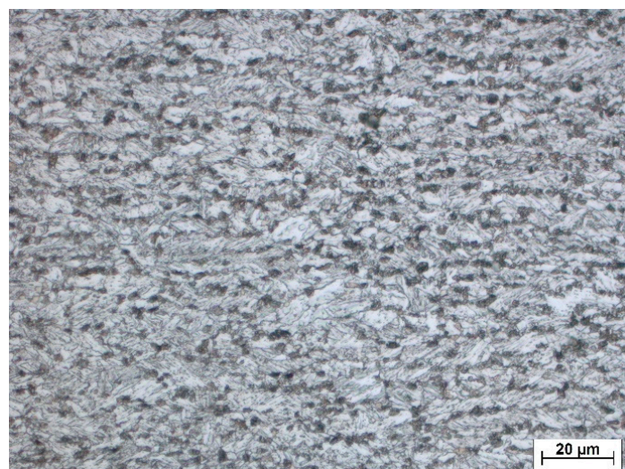
Figure 8. Microstructure of the inter-critical heat-affected zone (ICHAZ).
