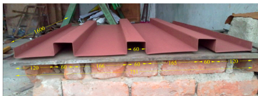
Figure 4. Rectangular profiled sheet (All dimensions are in mm).
