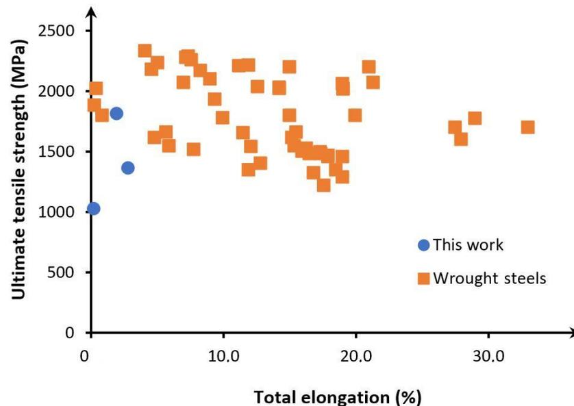
**Figure 19.** Chart showing ultimate tensile strength versus total elongation of the microstructures developed in this work against those reported for other wrought advanced bainitic steels [20,75–77,80].
