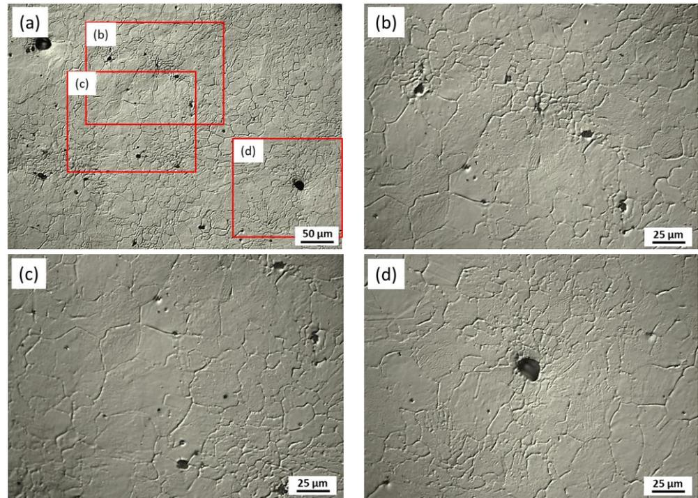
**Figure 4.** Light optical microscopy (LOM) micrographs of the prior austenite grain boundaries revealed by thermal etching. (a) Bright field image of the microstructure at a low magnification; (b–d) Micrograph corresponding to the red-square in image (a), using Nomarski microscopy (DIC).
