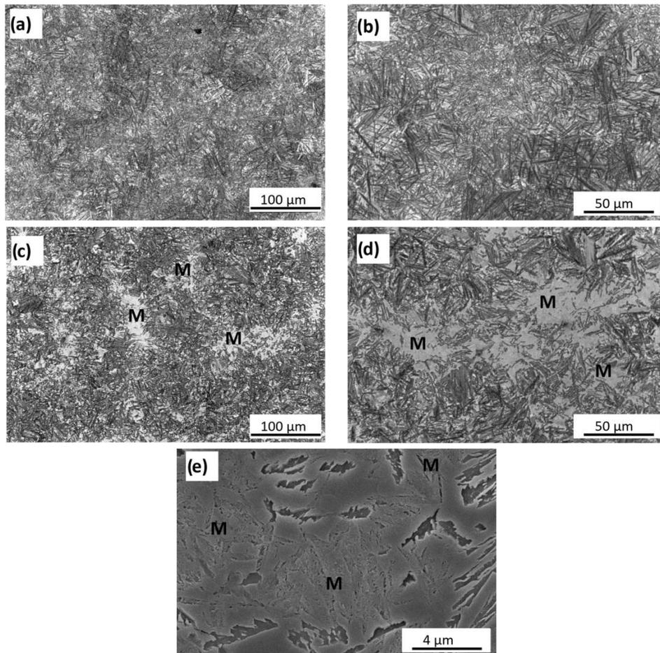
**Figure 16.** LOM and SEM micrographs showing the microstructure of a region near at the fracture surface of tensile samples after test, transformed at: (a,b) LOM-280 °C: No martensite was observed. (c,d) LOM-330 °C and (e) SEM-330 °C: Martensite can be appreciated, pointed out with M letter (lighter areas), evidencing the Transformation-Induced Plasticity (TRIP) effect. Nital 2%.
