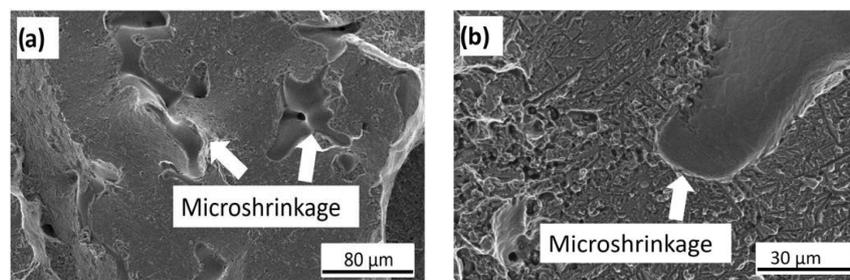
**Figure 15.** SEM micrographs showing casting defects in last to freeze zones (interdendritic regions) of fracture surface of tensile samples: (a) transformed at 280 °C, (b) transformed at 330 °C. Small black dots in Figure 13b corresponding to non-metallic inclusions.
