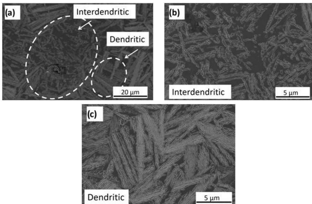
**Figure 10.** SEM micrographs showing: (a) the microstructure obtained at 330 °C for 360 min, (b) interdendritic and (c) dendritic regions. Nital 2%.
