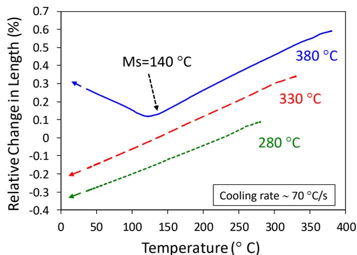
**Figure 12.** Dilatometric curves for the three isothermal temperatures, for 360 min of holding time. Relative change in length as function of temperature. Curves correspond to final stage of heat treatment (quenching) from the transformation temperature to room temperature.
