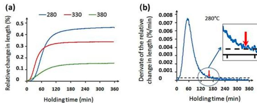
**Figure 6.** (a) Relative change in length function of time of isothermal heat treatments at 280, 330, and 380 °C. (b) Determination of time to end the transformation at 280 °C by means of the DRCL (horizontal line corresponds to 4% of the maximum DRCL and the arrow pinpointed the determined time).
