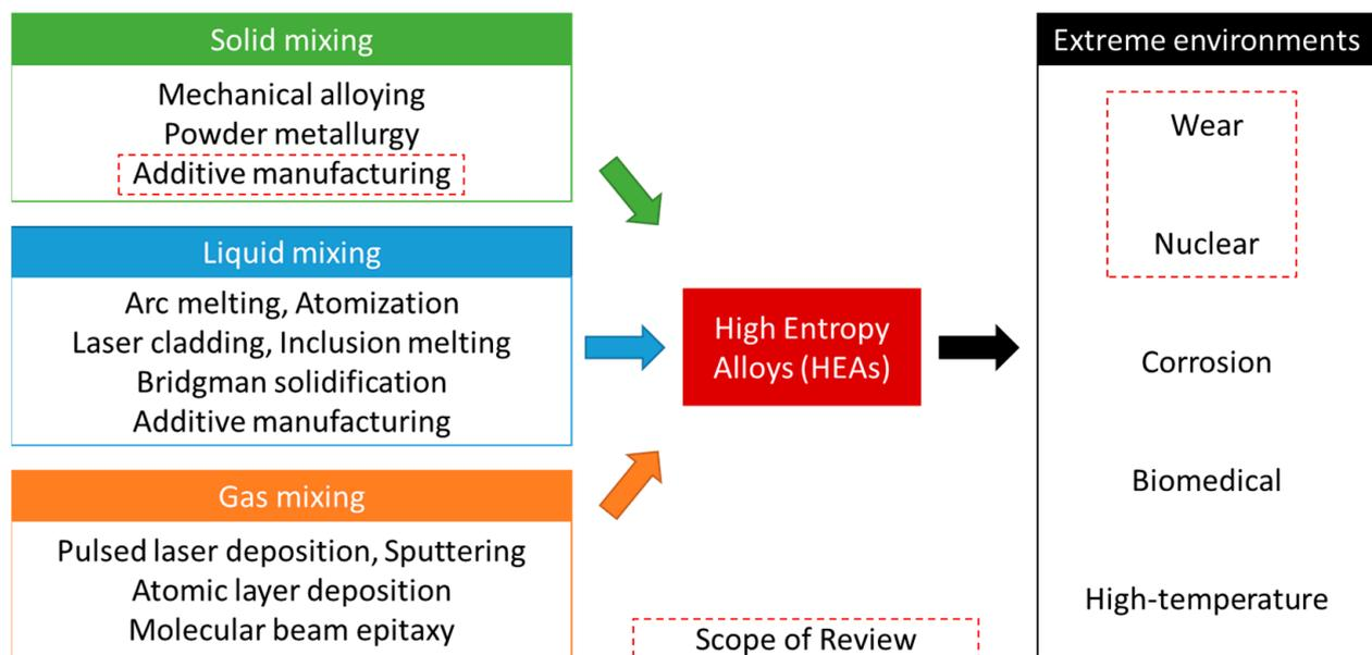
**Figure 2.** HEAs manufacturing methods and extreme environment applications. The scope of review includes recent advances in additive manufacturing of HEAs and their applications for wear-resistant and nuclear materials.
