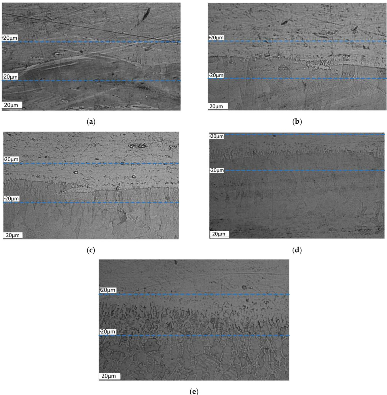
**Figure 2.** Microstructure of AlSi10Mg—SS316L bimetal interface zone: (a) SLM scanning mode 1, (b) SLM scanning mode 2, (c) SLM scanning mode 3, (d) SLM scanning mode 4, and (e) SLM scanning mode 5 (from bottom to top: a zone of deposited material, a heat-affected zone, and a substrate).
