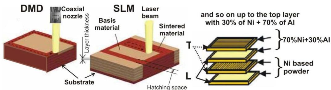
**Figure 1.** Obtaining the Functional graded structures by DMD and SLM methods Schematic of the multicomponent-graded structure fabrication by the DMD and SLM processes. Longitudinal, L; transversal, T [9].
