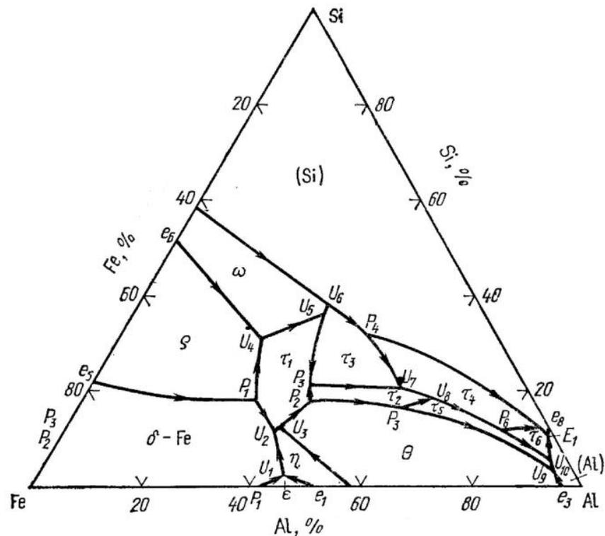
**Figure 3.** Fusibility diagram Fe-Al-Si (the percentage of elements is given by weight;  $\tau_1$ — $Al_3Fe_3Si_2$ ;  $\tau_2$ — $Al_{12}Fe_6Si_5$ ;  $\tau_3$ — $Al_9Fe_5Si_5$ ;  $\tau_4$ — $Al_3FeSi_2$ ;  $\tau_5$ — $Al_{15}Fe_6Si_5$ ;  $\tau_6$ — $Al_4FeSi$ ) data from [35].
