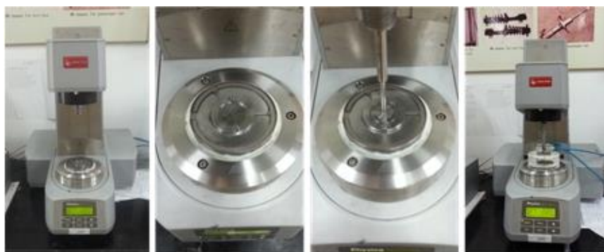
Figure 2. Experimental set-up and test process with MRC 301.
