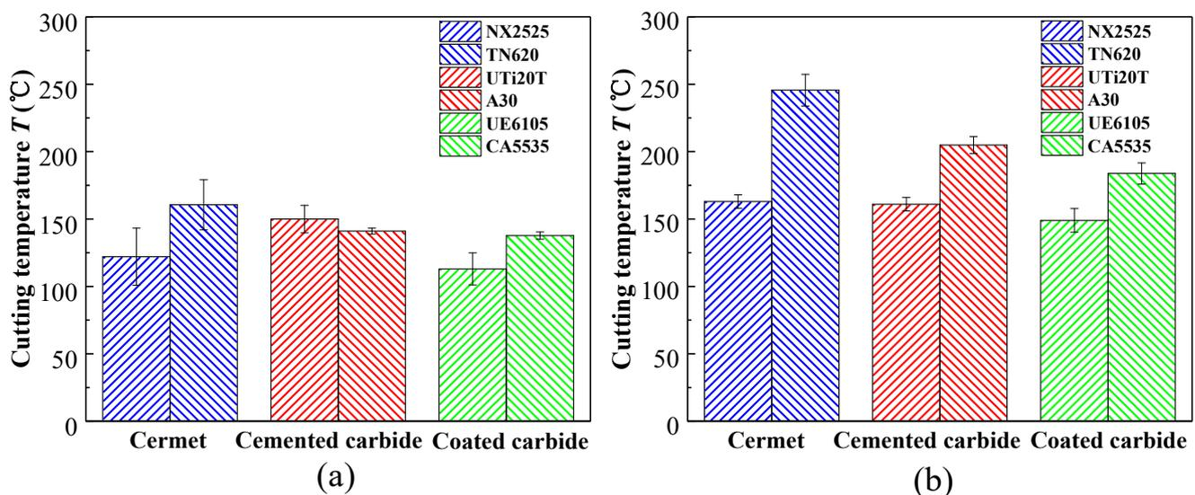
Figure 3. Cutting temperature for each tool at both cutting speeds: (a) 40 m/min and (b) 80 m/min.
