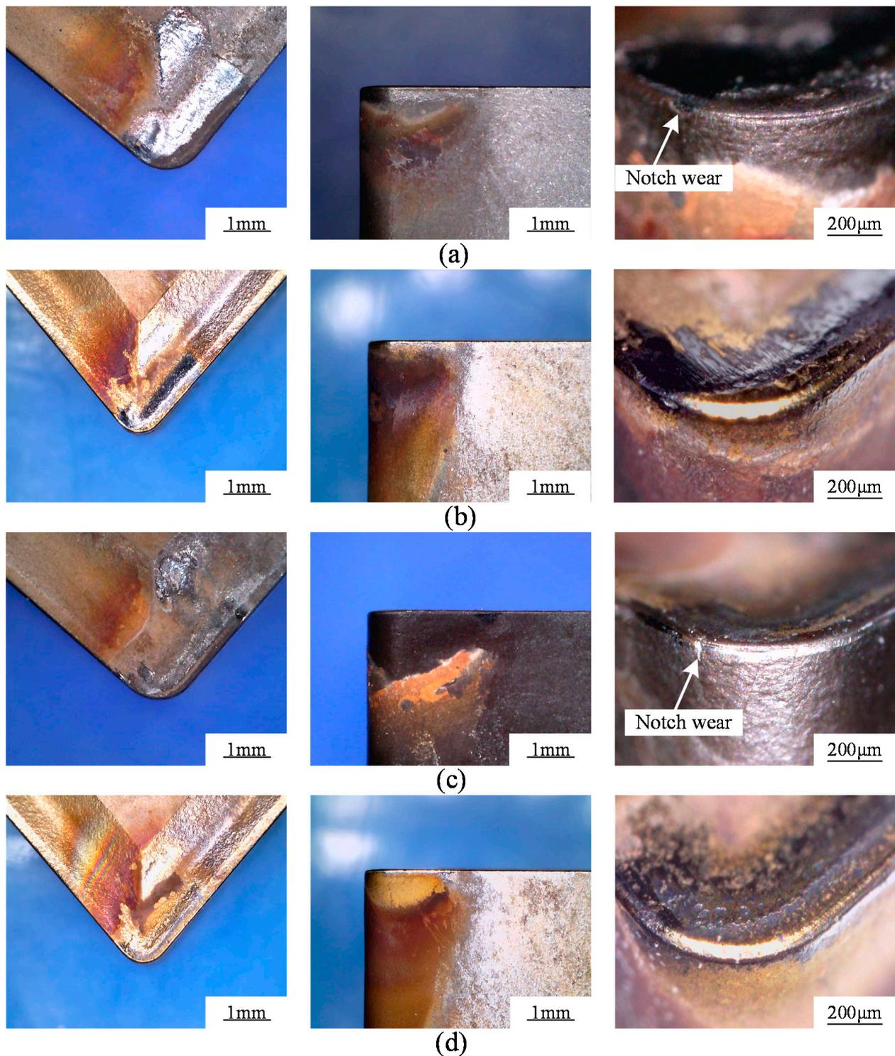
**Figure 6.** Wear morphologies of coated carbide tools at both cutting speeds: (a) UE6105 and (b) CA5535 at 40 m/min for 41 min, and (c) UE6105 and (d) CA5535 at 80 m/min for 15 min.
