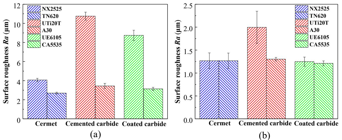
**Figure 7.** Surface roughness of machined workpieces obtained by each tool at both cutting speeds: (a) 40 m/min and (b) 80 m/min.
