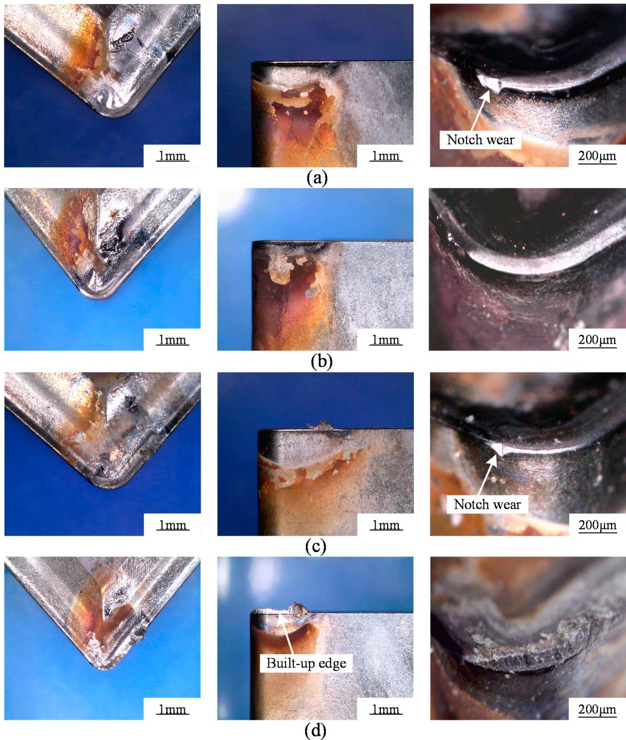
**Figure 4.** Wear morphologies of cermet tools at both cutting speeds: (a) NX2525 and (b) TN620 at 40 m/min for 41 min, and (c) NX2525 and (d) TN620 at 80 m/min for 15 min.
