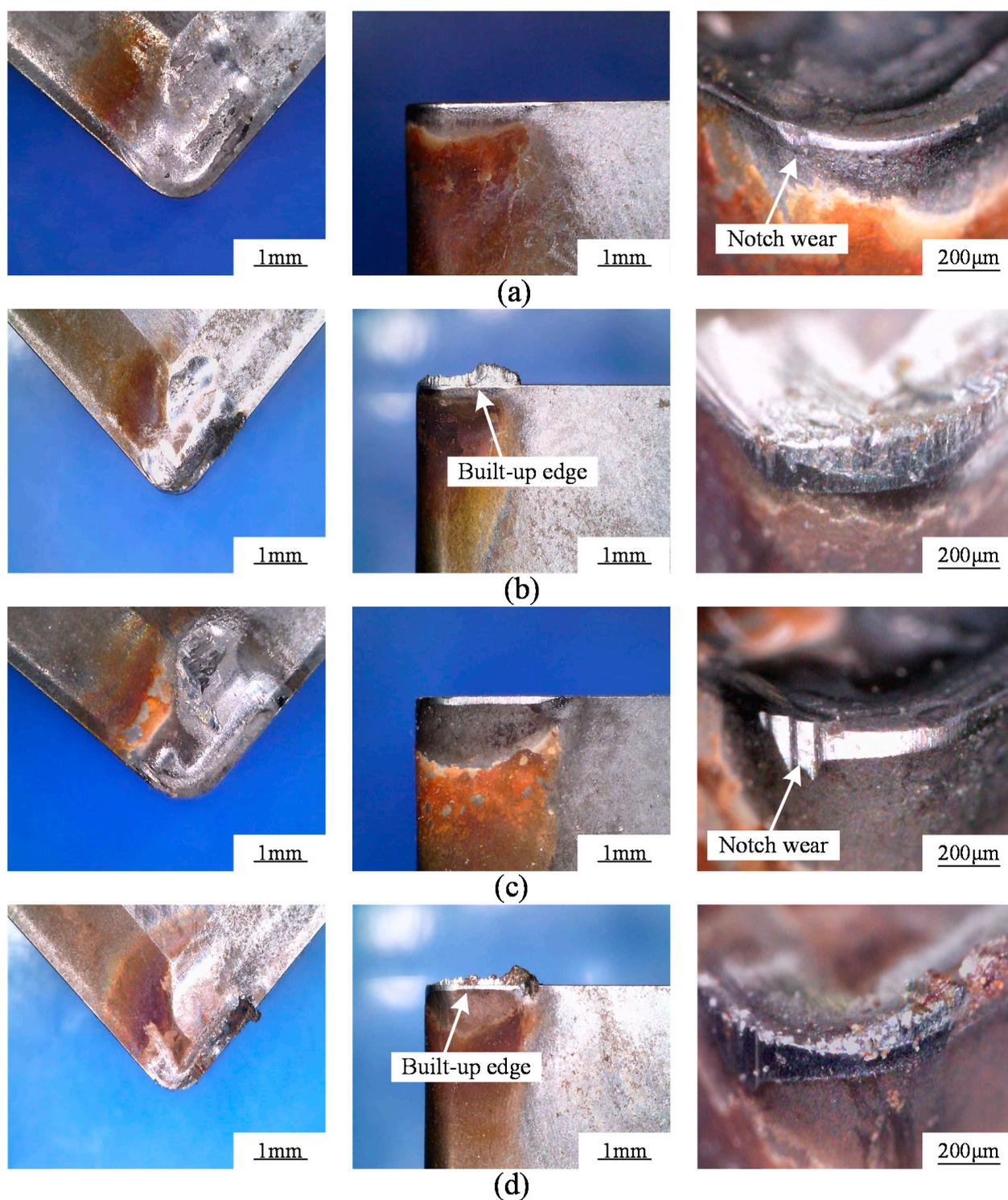
**Figure 5.** Wear morphologies of cemented carbide tools at both cutting speeds: (a) UTi20T and (b) A30 at 40 m/min for 41 min, and (c) UTi20T and (d) A30 at 80 m/min for 15 min.
