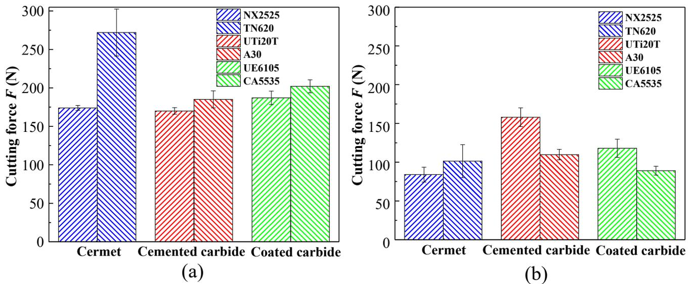
Figure 2. Cutting force for each tool at both cutting speeds: (a) 40 m/min and (b) 80 m/min.
