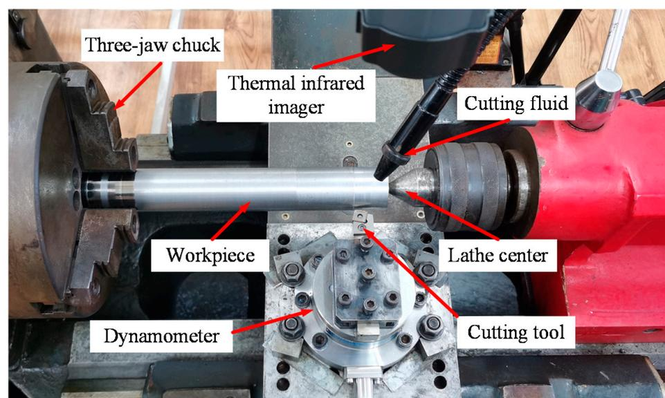
**Figure 1.** Photographic view of turning experiment.
