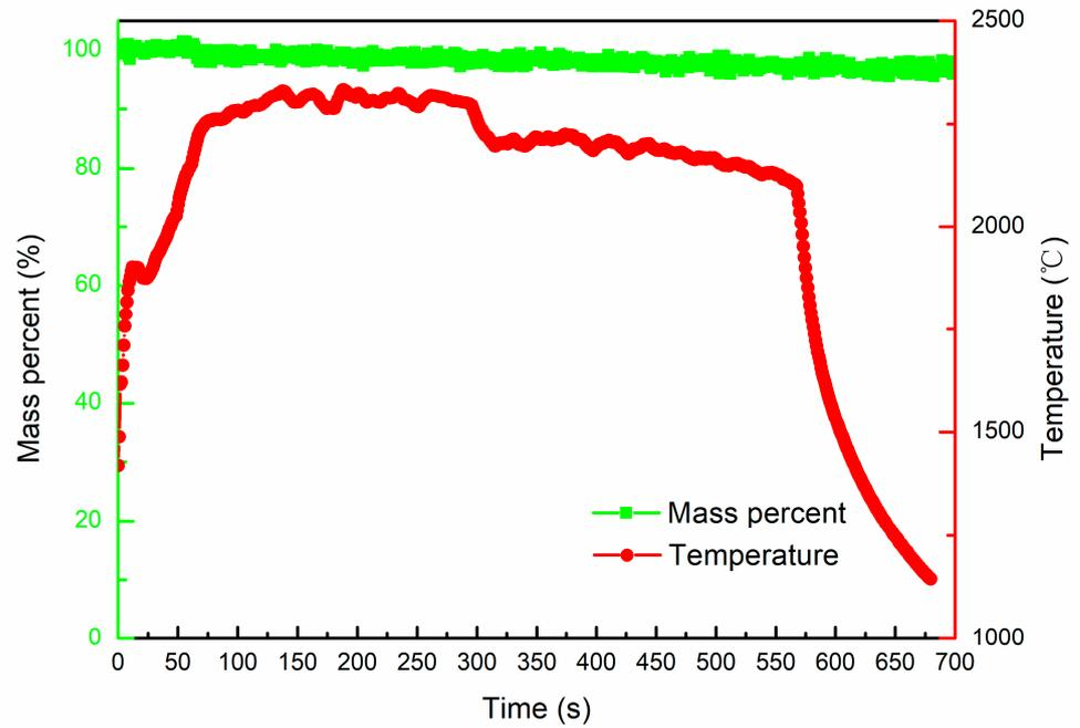
Figure 4. The vacuum evaporation of V by EBM.
