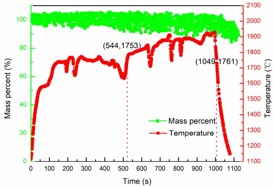
Figure 5. The vacuum evaporation of Al in Ti-Al alloy by EBM.
