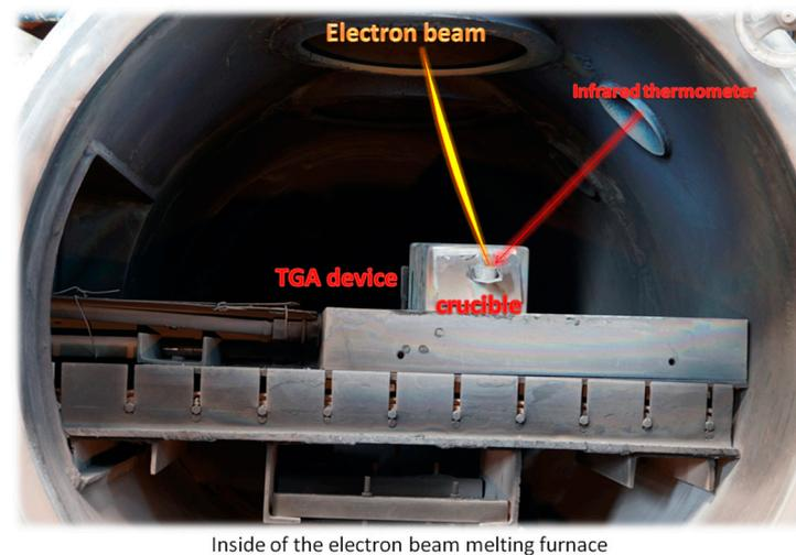
**Figure 1.** The actual setup and orientation of the TGA.
