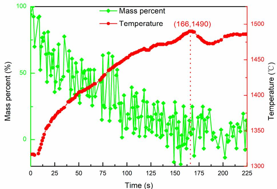
**Figure 2.** The vacuum evaporation of Al by EBM.
