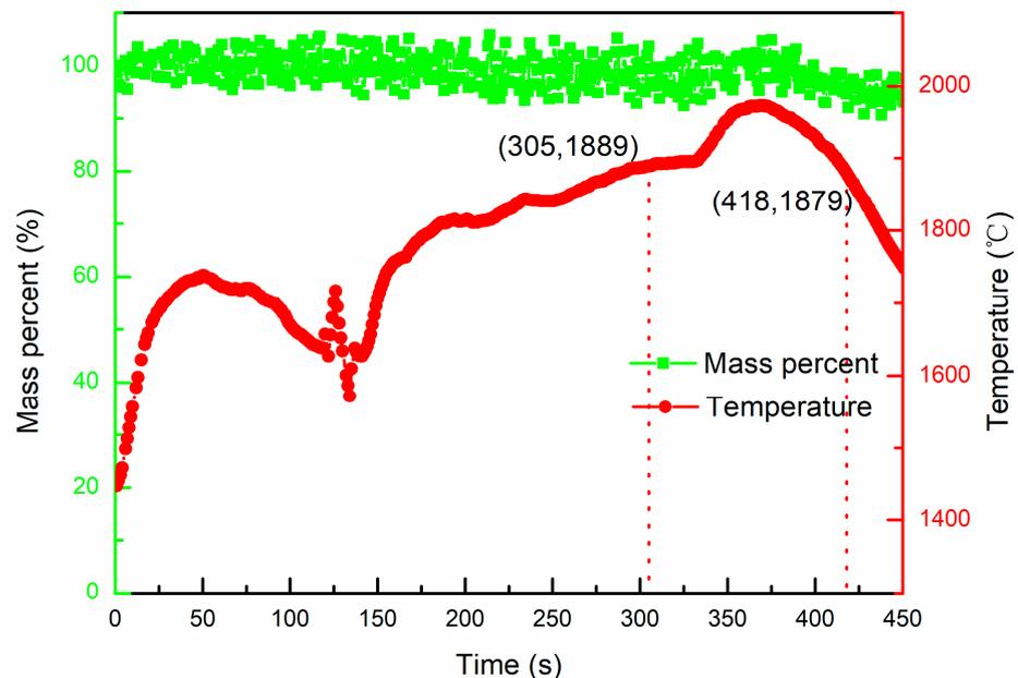
**Figure 7.** The vacuum evaporation of Al in TC4 alloy by EBM.
