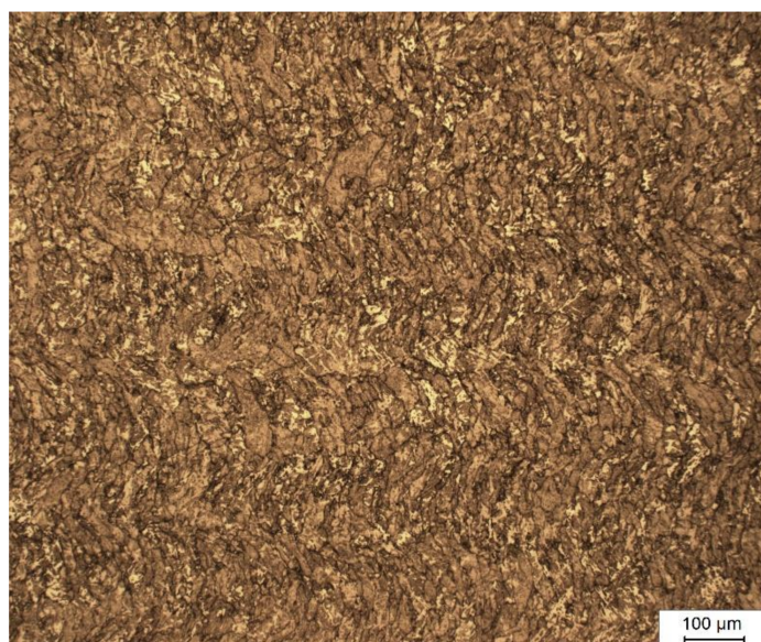
Figure 3. Optical micrograph of metallographic cross-section of PBF-EB processed X65MoCrWV3-2. Build direction is vertical. The main processing parameters were beam power 600 W, scan speed 3500 mm/s, and hatch distance 50 \mu\text{m} .
