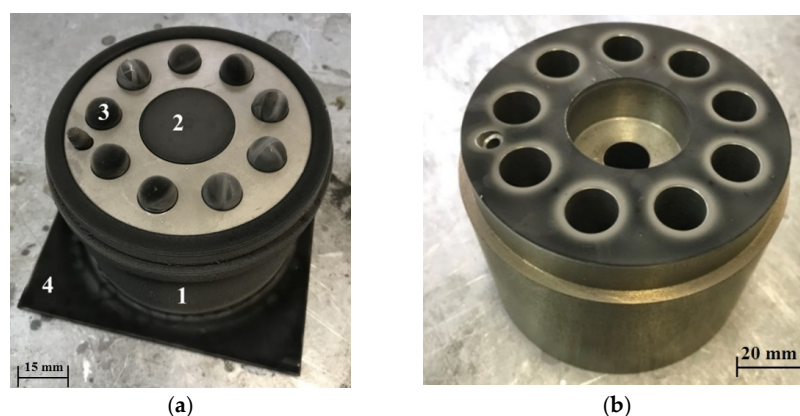
Figure 1. (a) Block blank in conventional tooling for ion-plasma nitriding; (b) block blank after ion-plasma nitriding (light gray zones with reduced hardness as a result of shielding from balls are clearly visible).
