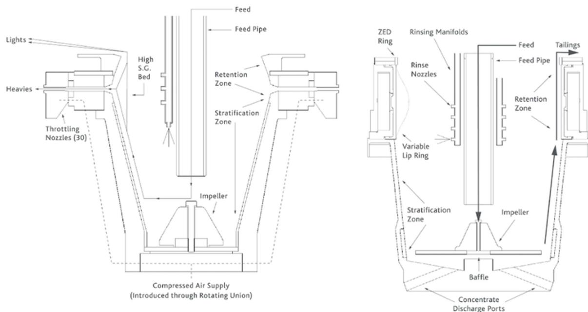
**Figure 3.** Cross sections of bowl of a continuous (left) and UF Falcon (right), adapted from [5].
