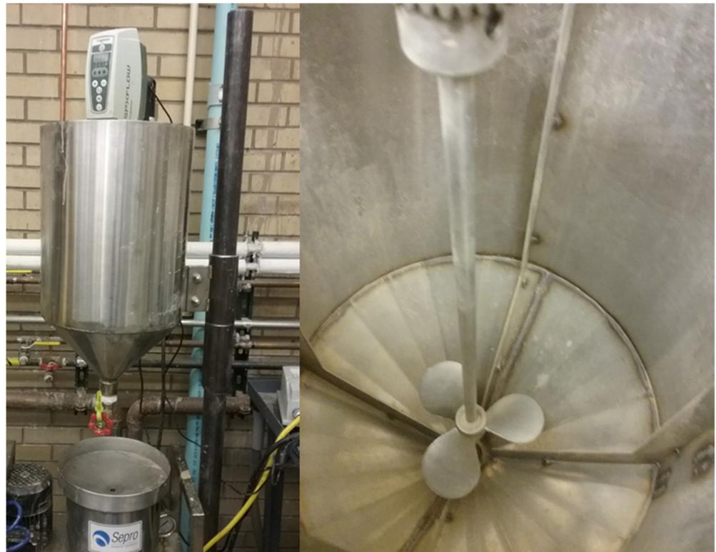
**Figure 9.** Feed tank, agitator, and laboratory Falcon optimal configuration as seen from the exterior (left) and interior (right).
