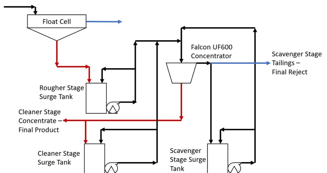
Figure 2. Replacement of TANCO gravity circuit with a single Falcon UF 600, recreated for legibility, adapted from [3,4].
