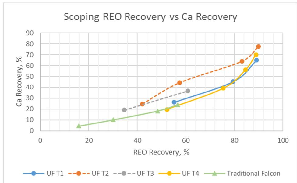
**Figure 8.** Scoping traditional and UF Falcon testing Ca recovery vs. REO recovery.
