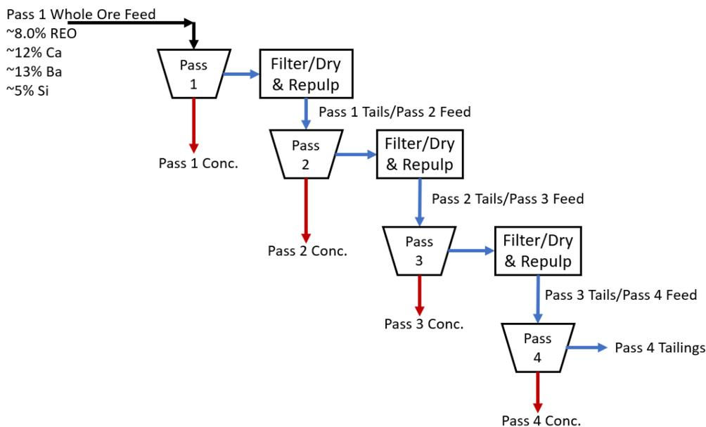
Figure 4. Generalized flowsheet of whole ore Falcon and UF Falcon testing. REO: rare earth oxide.
