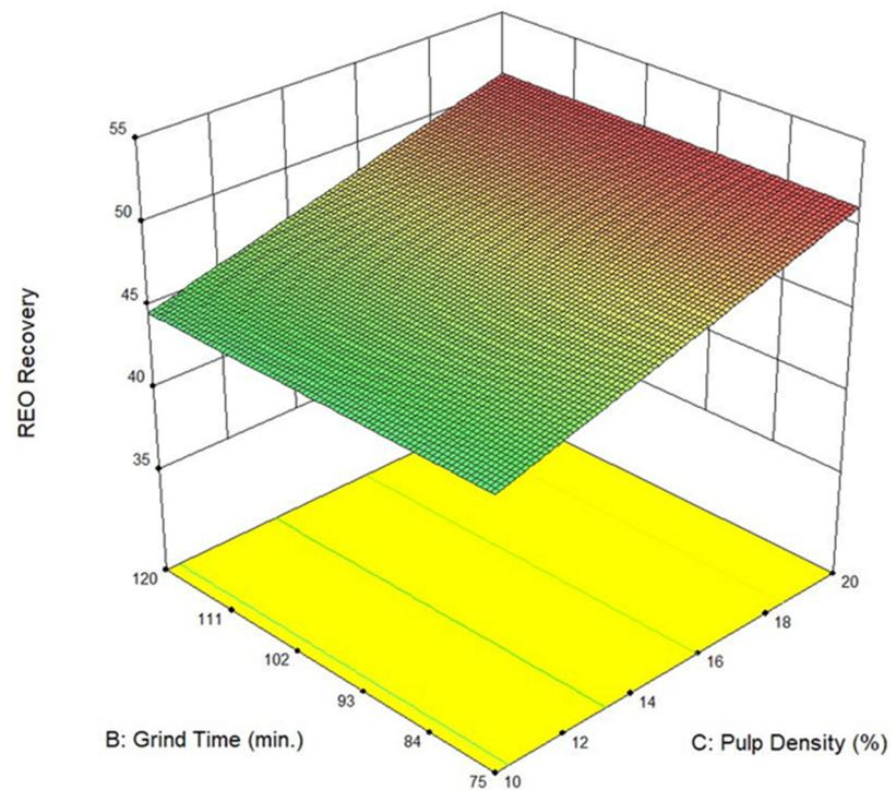
Figure 10. Predicted REO Recovery for Pass 1 UF Falcon tests at 1152.3 RPMs.
