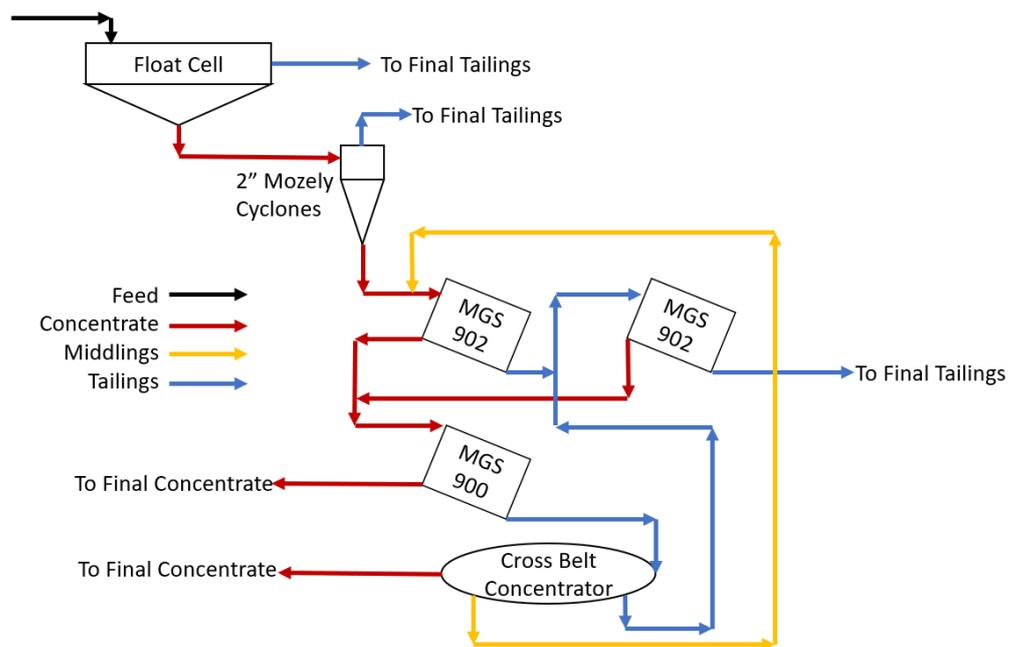
Figure 1. Original TANCO tantalum gravity circuit, recreated for legibility, adapted from [3,4].
