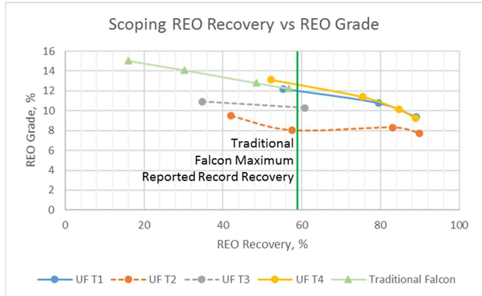
**Figure 7.** Scoping traditional and UF Falcon REO Grade/Recovery results. Tests shown with dashed lines indicate artificially poor performance due to suboptimal ancillary equipment. Overlaid is the previous traditional Falcon REO recovery record, after 3 passes, of 59.2%, as set by Schriener [5,6].
