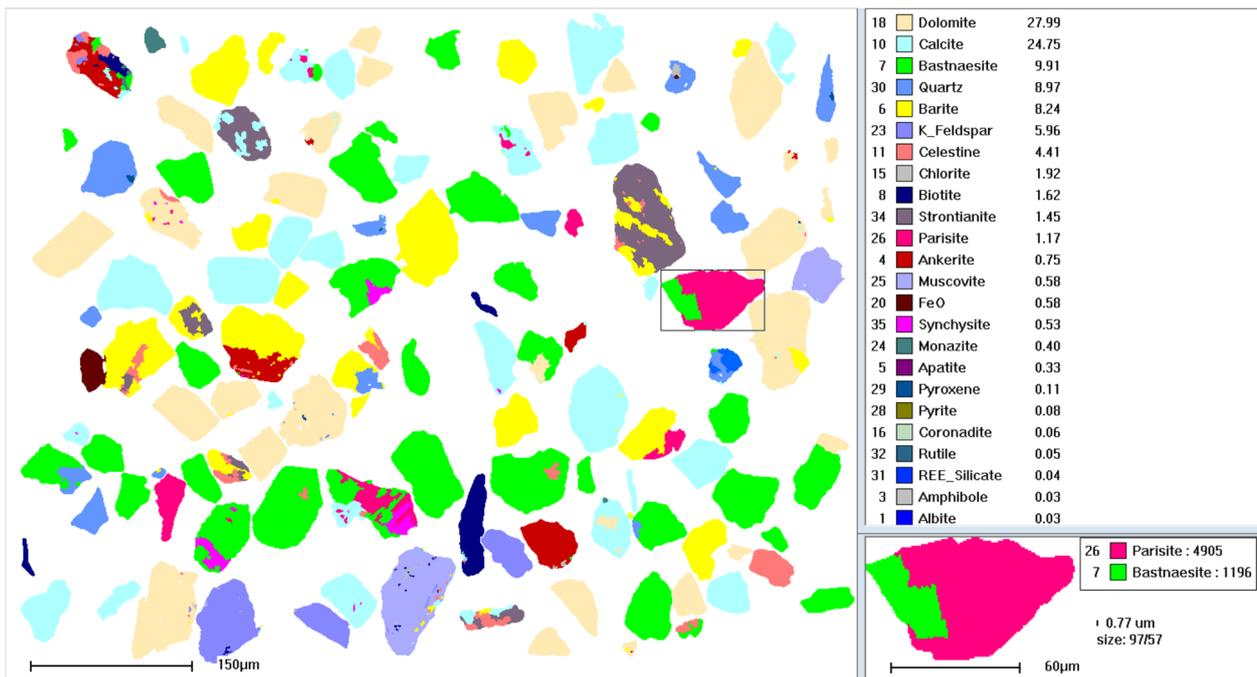
**Figure 6.** False-color image from MLA of the whole ore specimen. Values represent surface area percentages.
