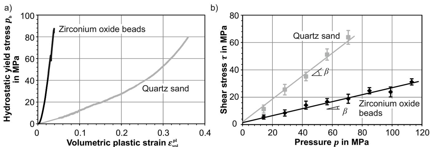
**Figure 12.** Yield stresses of quartz sand and zirconium oxide beads for (a) volumetric compression and (b) under shear loading, according to [20].
