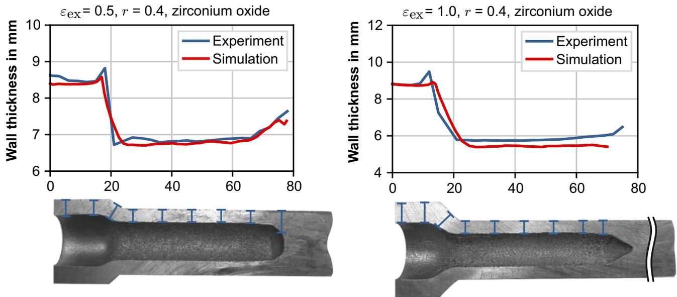
**Figure 17.** Wall thicknesses measured in experiments and obtained by process simulations.
