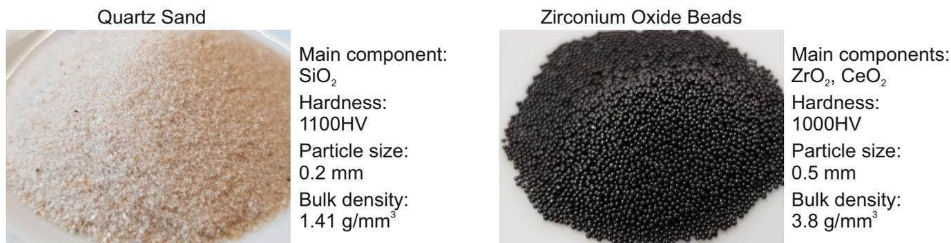
**Figure 11.** Granular media used as lost cores in cold forging.
