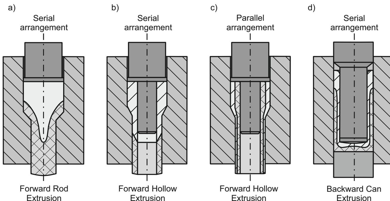
**Figure 1.** Cold forging processes and arrangement of materials in used composite billets. (a–c) representing works by Gumm [1] and (d) investigations by Wagener and Haats [4].
