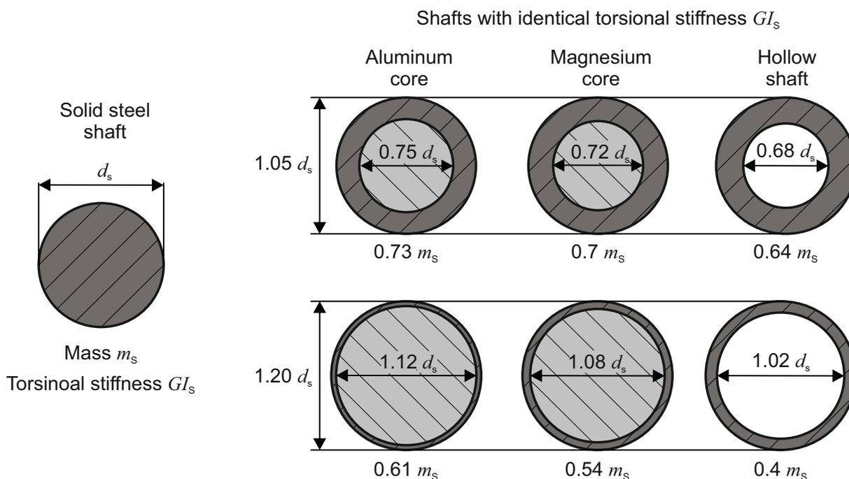
**Figure 18.** Mass savings for substituting a solid steel shaft by composite shafts with aluminum core, magnesium core and hollow shafts with identical torsional stiffness.
