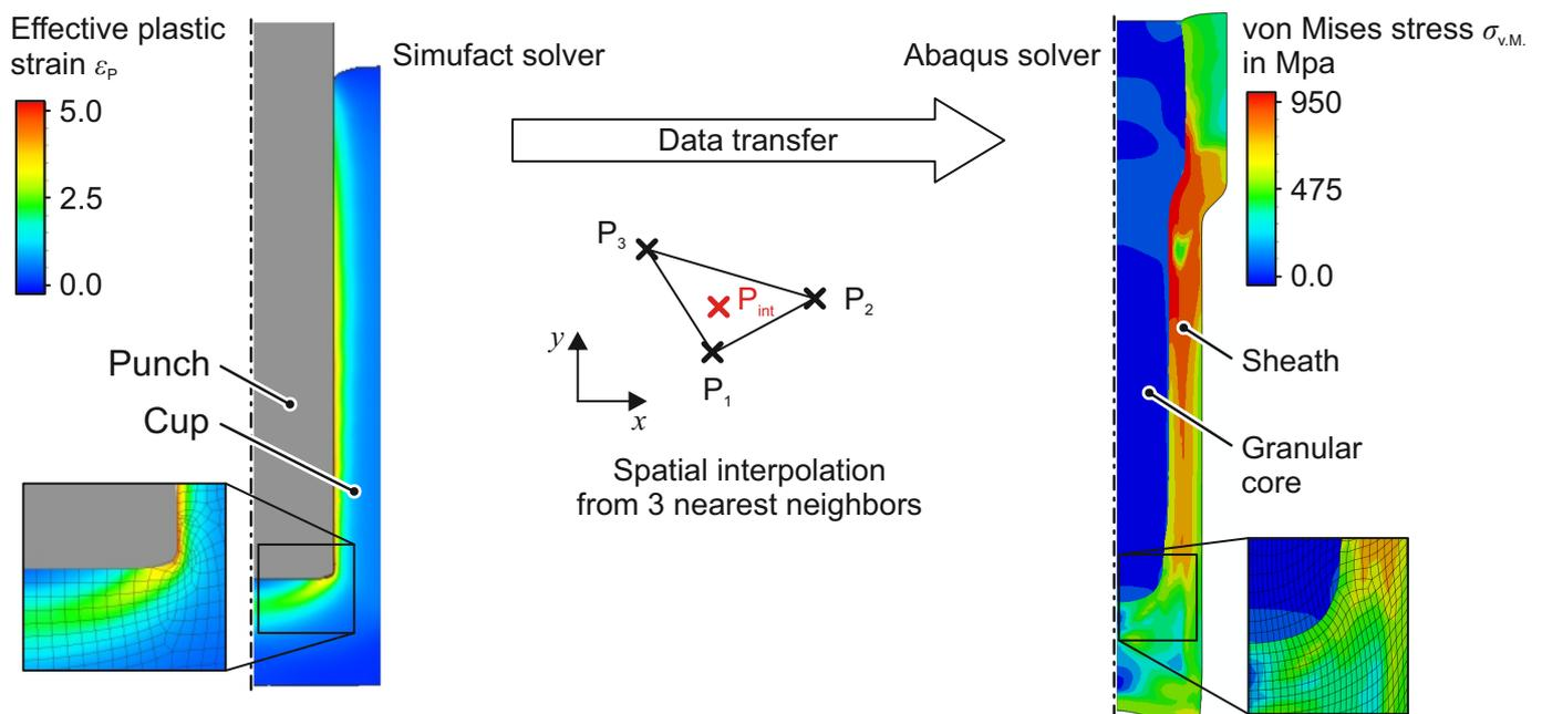
**Figure 15.** Simulation model for the process chain of cold forging with granular medium based cores. Backward can extrusion is modelled using Simufact forming. The process step of forward rod extrusion is modelled using Abaqus. The data transfer between the two solvers is implemented by a Python script.
