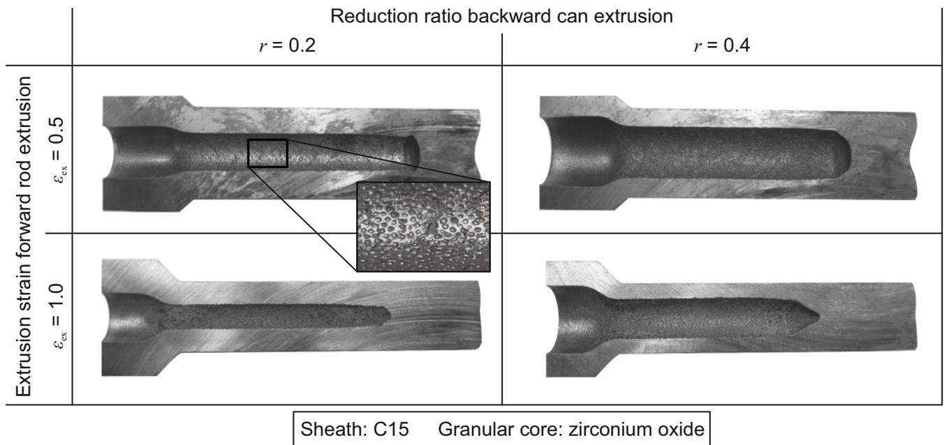
**Figure 13.** Hollow shafts produced by forward rod extrusion of steel cup billets filled with zirconium oxide, cut open to reveal inner surface.
