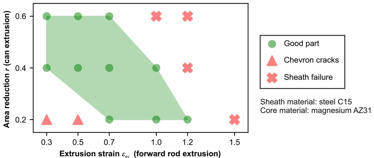
Figure 7. Process window of magnesium-steel composite forward rod extrusion.
