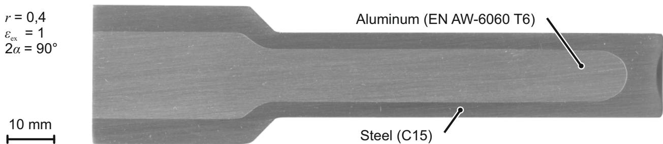
**Figure 2.** Composite shaft, produced by forward rod extrusion of a backward can extruded steel shaft with an aluminum core, according to [9].
