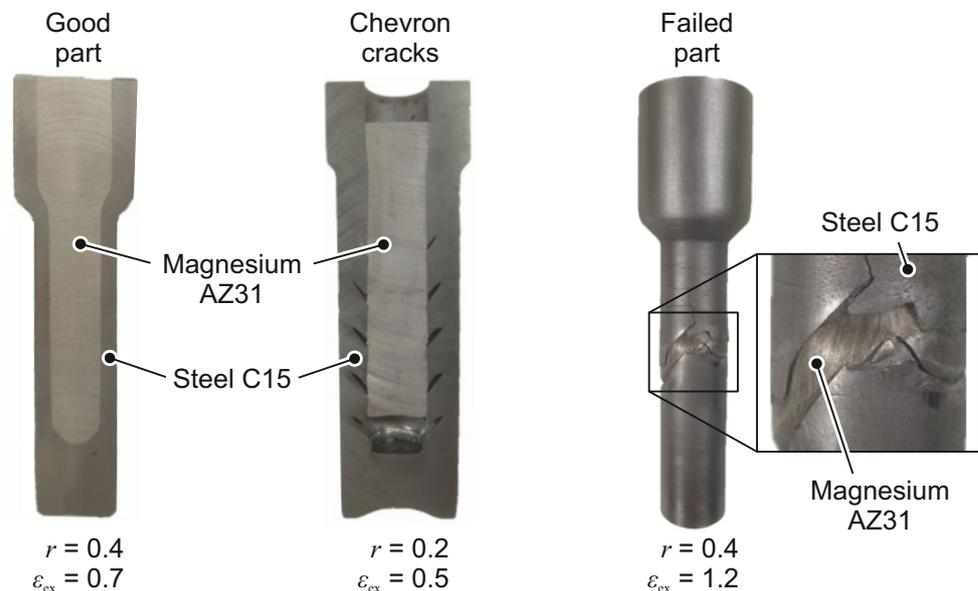
Figure 5. Parts produced by magnesium-steel composite forward rod extrusion.
