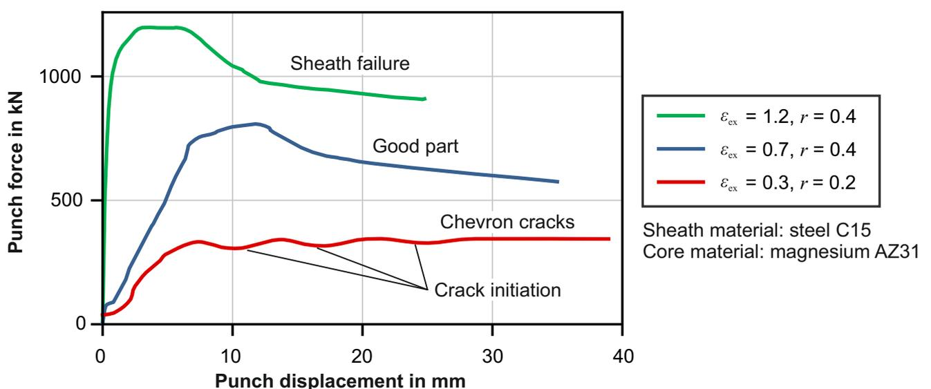
Figure 6. Punch forces in magnesium-steel composite forward rod extrusion.
