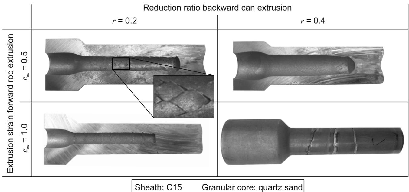
**Figure 14.** Hollow shafts produced by forward rod extrusion of steel cup billets filled with quartz sand, cut open to reveal inner surface.
