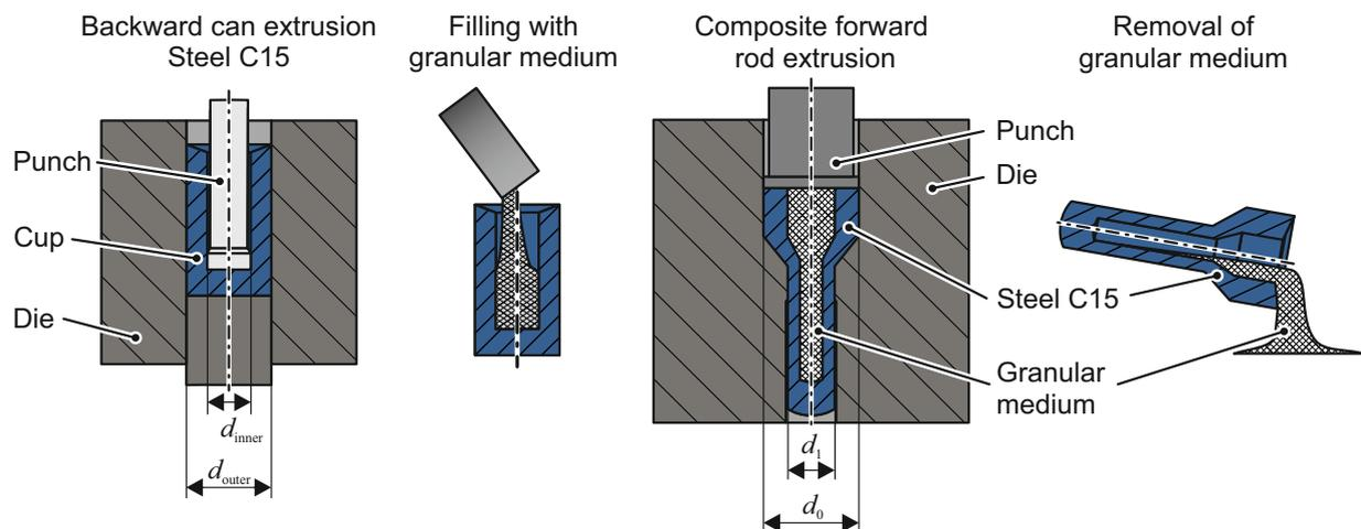
**Figure 10.** Process route for production of hollow shafts by means of cold forging with granular media.
