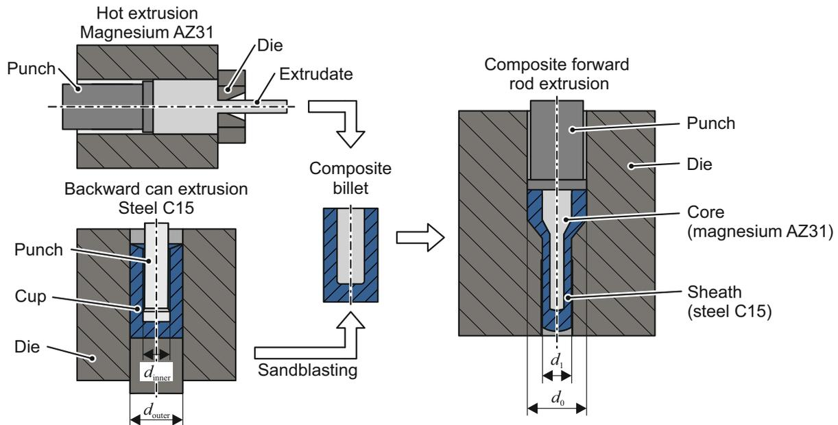
**Figure 4.** Process route for production of composite shafts with magnesium core. The composite core, consisting of a backward can extruded steel cup and a hot extruded magnesium core is formed to a shaft by composite forward rod extrusion.
