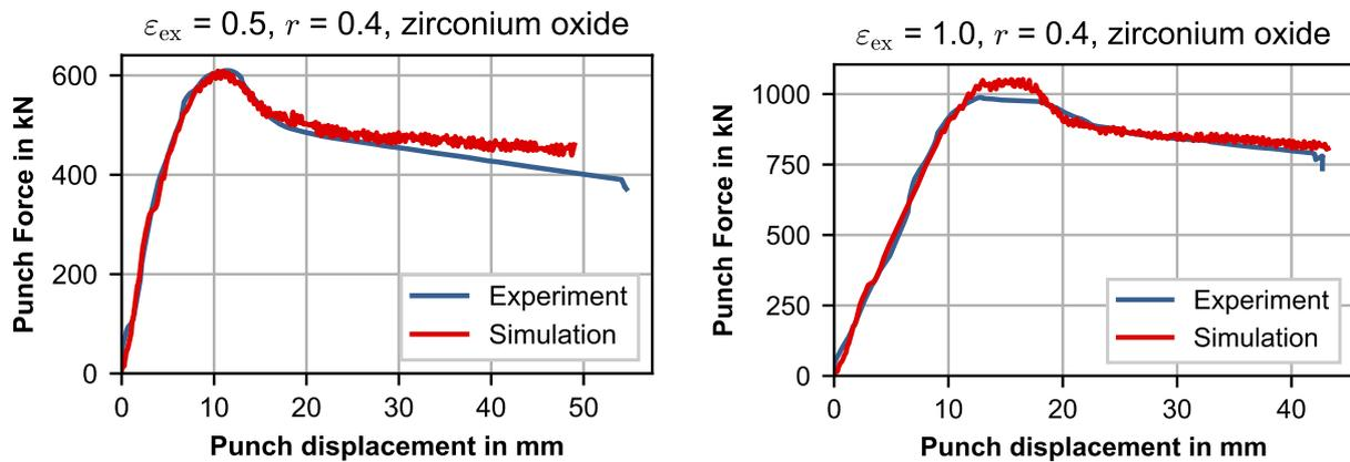
**Figure 16.** Punch force measured in experiments and obtained from simulation of forward rod extrusion with zirconium oxide core.
