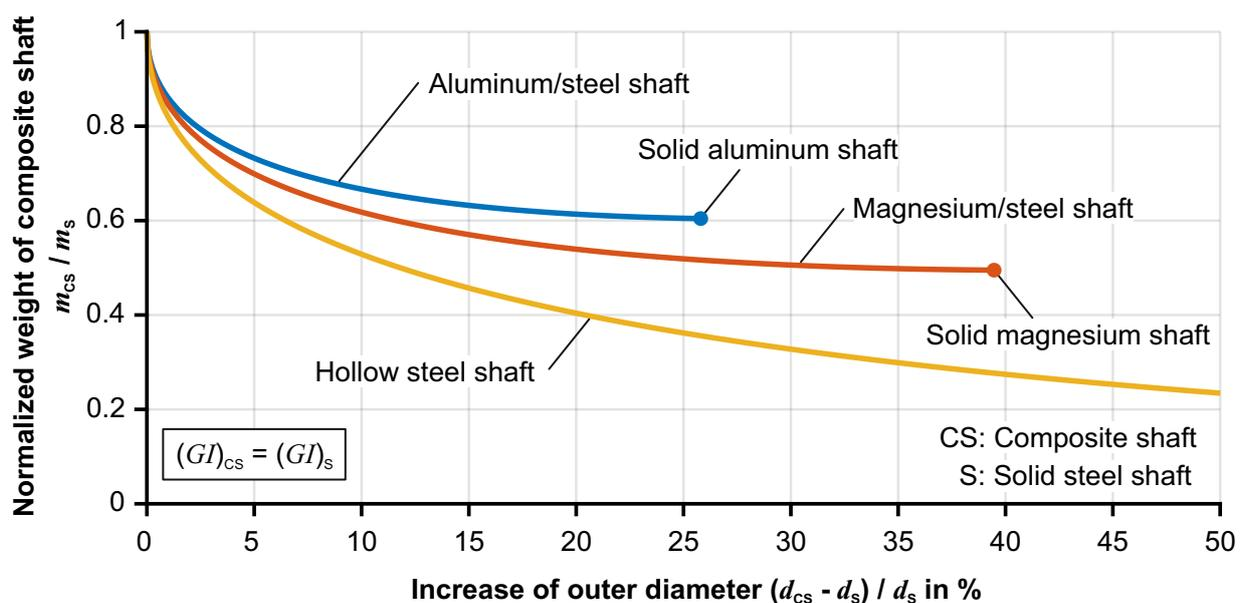
**Figure 3.** Mass savings for substituting a solid steel shaft by composite shafts with aluminum core, magnesium core and hollow shafts with identical torsional stiffness.
