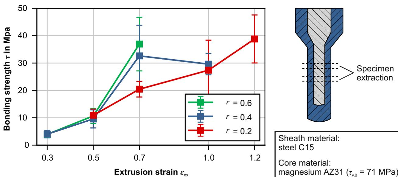
Figure 9. Bond strength of magnesium core and steel sheath, obtained by push-out testing and location of specimen extraction.
