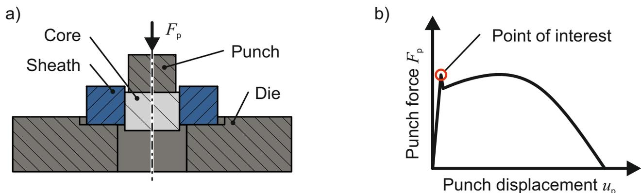
Figure 8. Principle of push-out testing: (a) tool set up and (b) evaluation of obtained force-displacement-curve.
