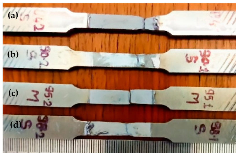
Figure 10. Fracture locations of the joints welded in different cooling conditions (a) NAC. (b) S-RM (c) S-IM (d) C-RJ.
