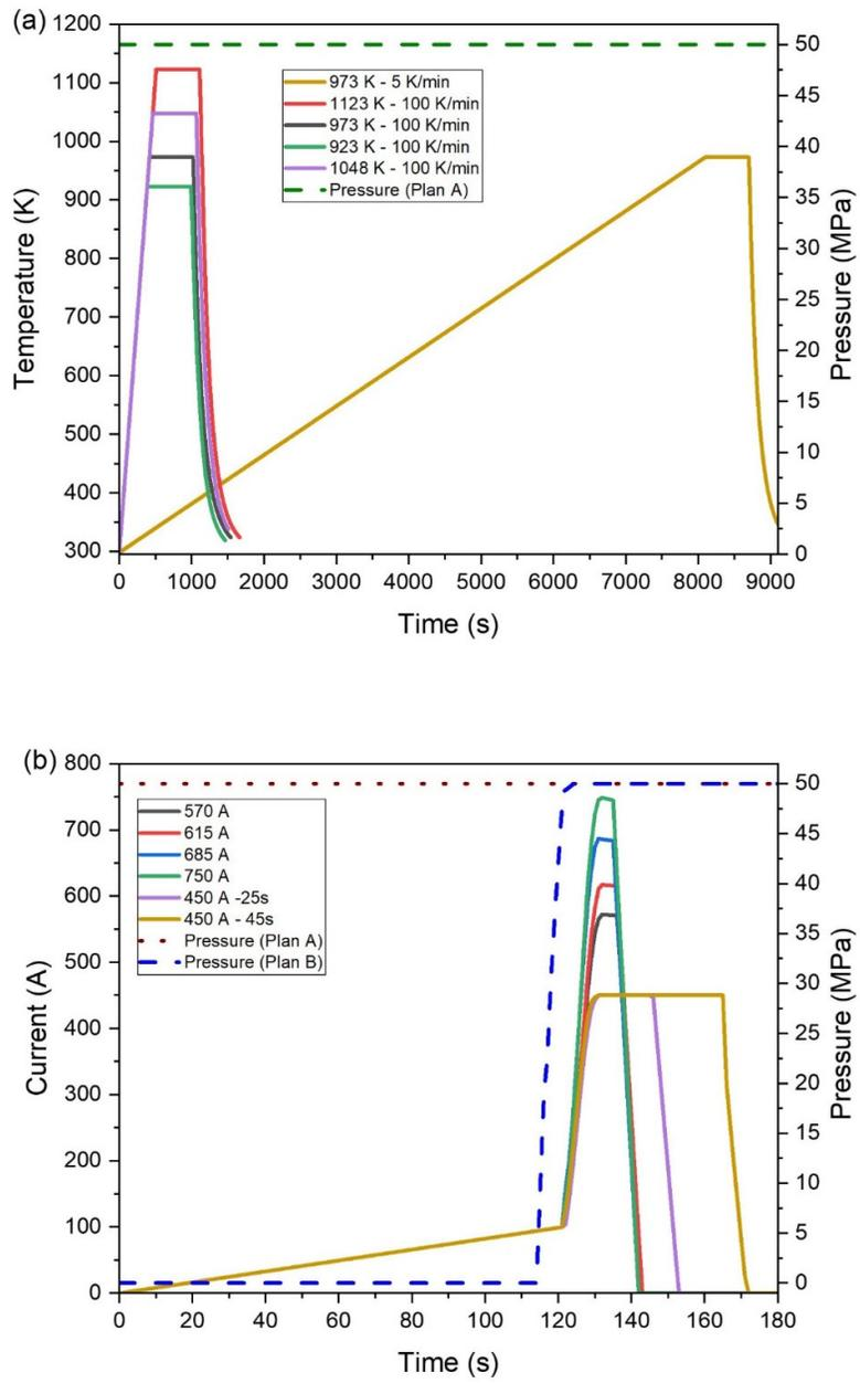
**Figure S1.** Sintering profiles for different consolidation schemes: (a) SPS; (b) FSPS Sintering conditions for different consolidation schemes.
