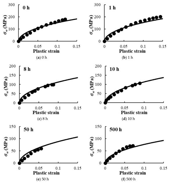
**Figure 7.** Comparison of the work hardening behaviour of AA2198 with different artificially aged states (time) at 155 °C from experiments (symbols [34]) and modelling results from Table 3 (lines): (a) not-aged; (b) 1h aged; (c) 8h aged; (d) 10h aged; (e) 50h aged and (f) 500h aged.
