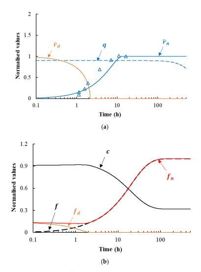
**Figure 5.** Comparison of evolutions of indicated microstructural variables during artificial ageing of AA2198 at 155 °C from experiments (symbols [35]) and modelling results from Table 3 (lines). (a) Variables of dimensions of precipitates; (b) Variables of volume fractions and solid solution.
