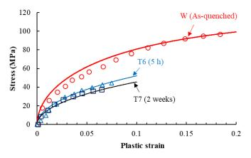
**Figure 4.** Comparison of the work hardening behaviour of AA6063 with different artificially aged states (time) at 185 °C from experiments (symbols [33]) and modelling results from Table 1 (lines).
