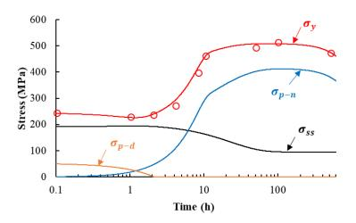
**Figure 6.** Comparison of evolutions of yield strength and corresponding strengthening components during artificial ageing of AA2198 at 155 °C from experiments (symbols [34]) and modelling results from Table 3 (lines).
