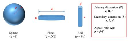
Figure 1. Summary of key dimensions of general precipitates.
