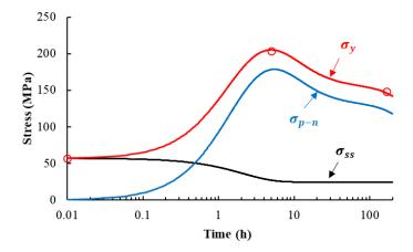
**Figure 3.** Comparison of evolutions of yield strength and corresponding strengthening components during artificial ageing of AA6063 at 185 °C from experiments (symbols [33]) and modelling results from Table 1 (lines).
