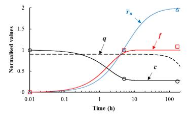
**Figure 2.** Comparison of evolutions of indicated microstructural variables during artificial ageing of AA6063 at 185 °C from experiments (symbols [33]) and modelling results from Table 1 (lines).
